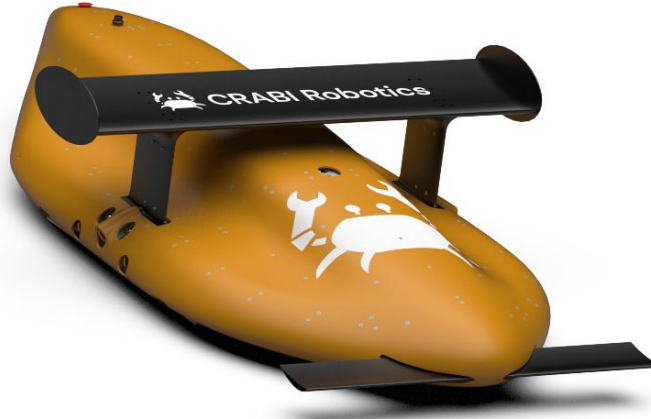
Fig.5: Grooming platform: hydrodynamic body with inverted main wing and forward canards providing the speed-dependent downforce of Section 4. Hull-facing equipment is not shown.
