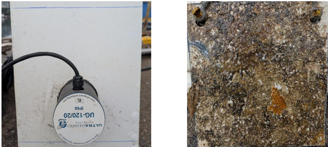
Fig.4: Test panels after two months of exposure to biofouling in Perth, Australia. Both panels were coated by an aliphatic acrylic polyurethane paint; the panel on the left was additionally exposed to ultrasound throughout the test.
