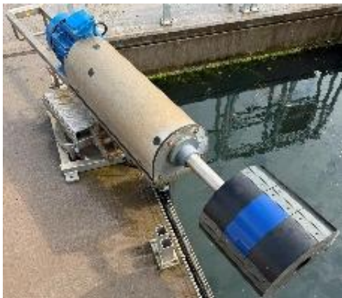
Fig.1: a) CoaST Maritime Test Centre (CMTC) in the Baltic Sea, b) rotor set-up for dynamic exposure and c) set-up for static exposure in natural sea water
