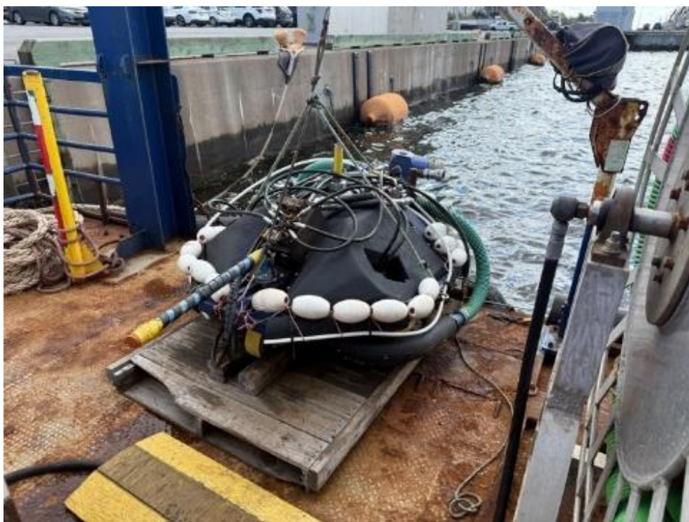
Fig.1: Remora Hull Cleaning Vehicle awaiting deployment, Credit: Subsea Global Solutions
