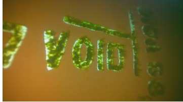
Marking paint failure
