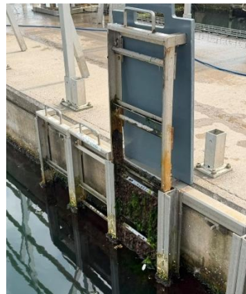
Fig.1: a) CoaST Maritime Test Centre (CMTC) in the Baltic Sea, b) rotor set-up for dynamic exposure and c) set-up for static exposure in natural sea water
