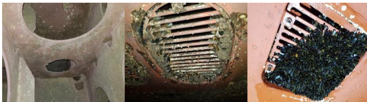
Fig.1: Examples of biofouling inside sea chests and on gratings applied following normal yard application practices and with an antifouling product from the main hull
