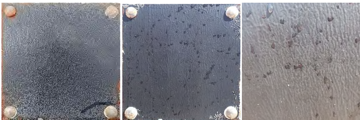
Coat.4 – initial biofouling after 3 weeks – cleaned - Close-up shows no visible damages.
