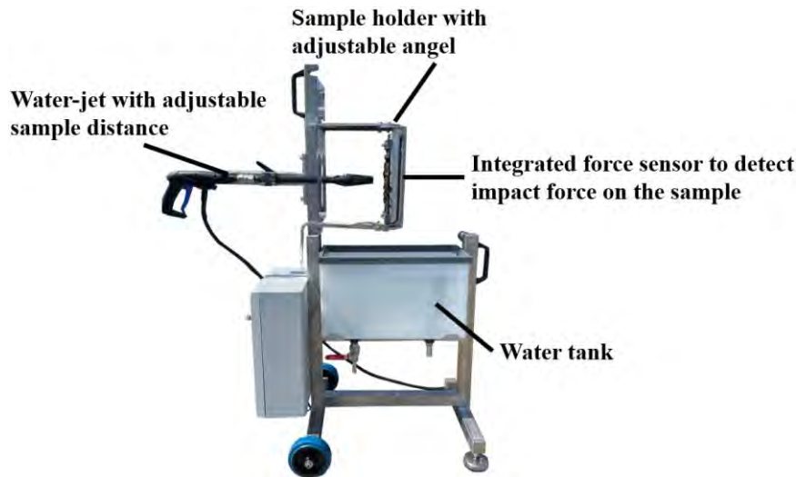
Fig.4: In-water water-jet cleaning device with adjustable nozzle angle and distance to sample surface
