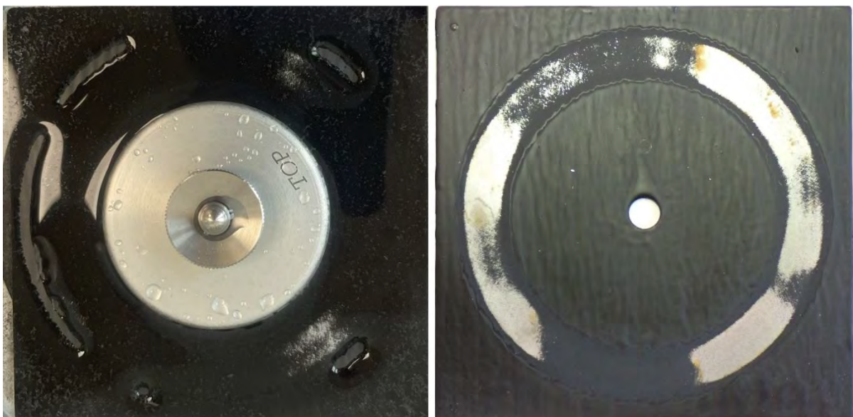
Fig.8: The wet tested Coat.4 test panel after 619 cycles (left, still wet) and 784 cycles (right, dried) in the Taber Abraser. At measuring points B, C, D, E, F, I, J, and K, the coating was completely worn away. These abraded points were not included in the mean values.
