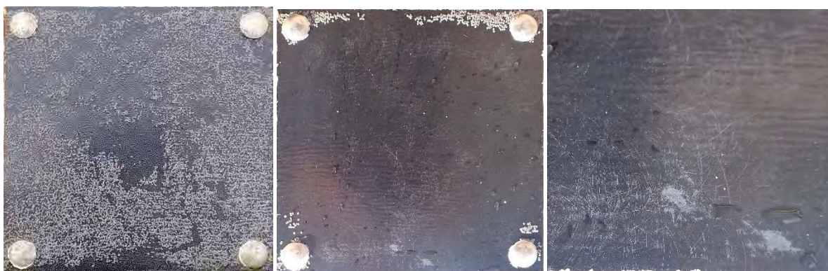
Coat.5 – initial biofouling after 3 weeks – cleaned - Close-up shows a lot of circular scratches and abrasion caused by detritus of the small barnacles.
