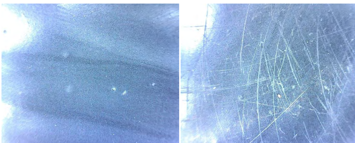
Coat.5 – surface after cleaning without biofouling (left) and with initial biofouling (right): Deep scratches visible.
