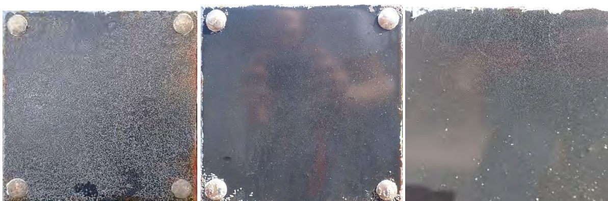
Coat.8 – initial biofouling after 3 weeks – cleaned - Close-up shows a lot of circular scratches caused by detritus of the small barnacles.
