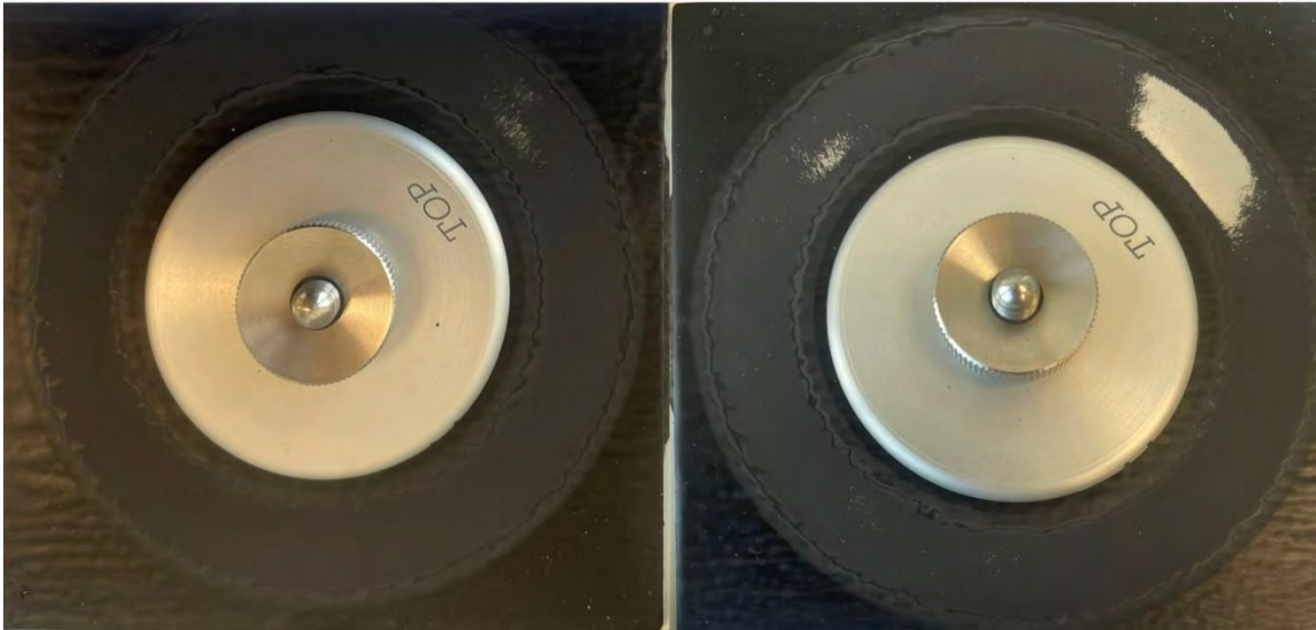
Fig.7: The dry tested Coat.4 test panel after 729 cycles (left) and 912 cycles (right) in the Taber Abraser. At measuring points B and C, the coating was completely worn away. These points were not included in the mean values.
