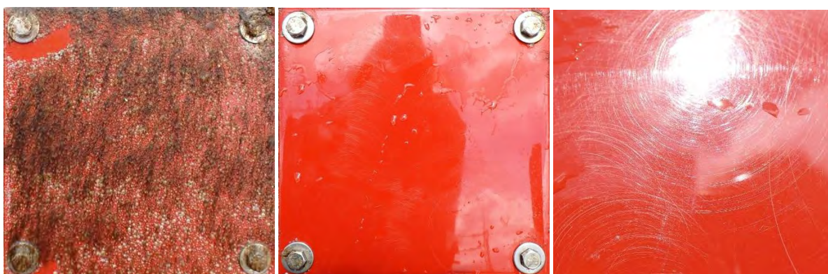
Coat.9 – initial biofouling after 4 weeks – cleaned - Close-up shows a lot of circular scratches caused by detritus of the small barnacles.
