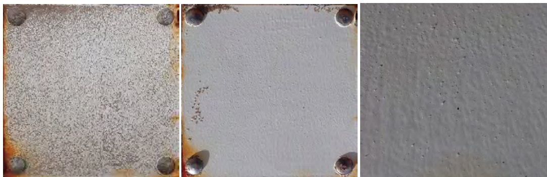
Coat.3 – initial biofouling after 3 weeks – cleaned - Close-up shows no visible damages.
