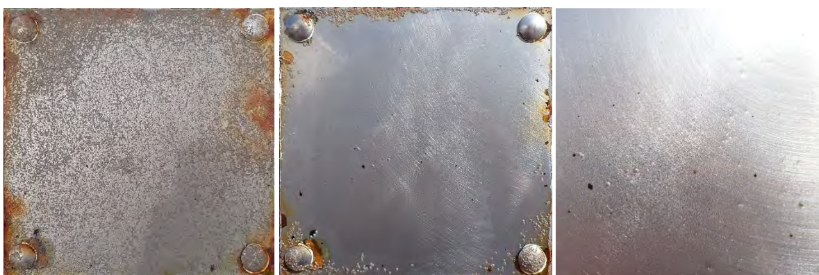
Coat.6 – initial biofouling after 3 weeks – cleaned - Close-up shows circular scratches caused by detritus of the small barnacles.
