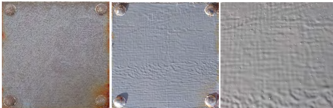
Coat.2 – initial biofouling after 3 weeks – cleaned - Close-up shows no visible damages.
