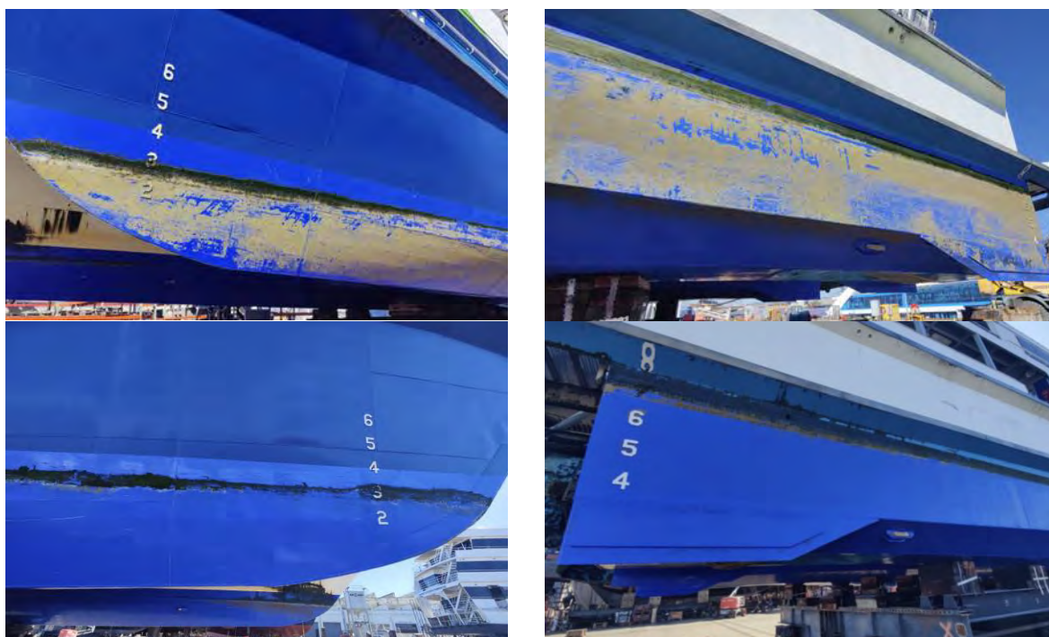
Fig.5: Side-by-side hull fouling after one month in San Francisco Bay. One side cleaned just before haul-out, the other not cleaned for a month.
