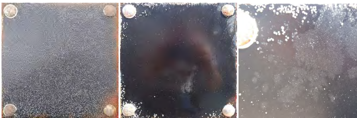
Coat.7 – initial biofouling after 3 weeks – cleaned - Close-up shows abrasion.
