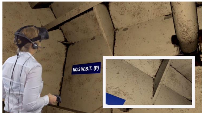
Fig.5: Vision of drone-based images mapped on 3D model and viewed in VR, Cabos et al. (2017)
