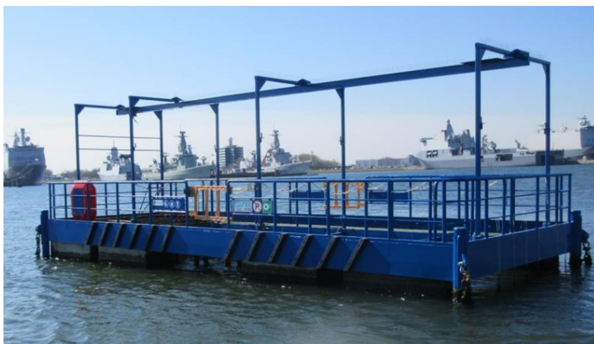
Fig.1: Raft exposure facility of Endures in the harbour of Den Helder, The Netherlands
