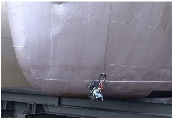
Fig.6: Crawler traversing the bow of the boat. As shown, the crawler is able to drive over the curvature even hanging upside down, and therefore move from one side of the ship to the other with only minor difficulties.
