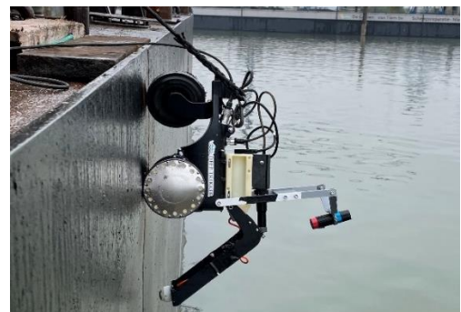
Fig.2: Magnetic crawler vertically sitting on a ship hull. The sensor and mount are attached to the crawler, with an overhead camera attached to provide documentation of the measuring process. Further, the crawler is connected to the remote via tether cable and an additional safety rope as a precaution.
