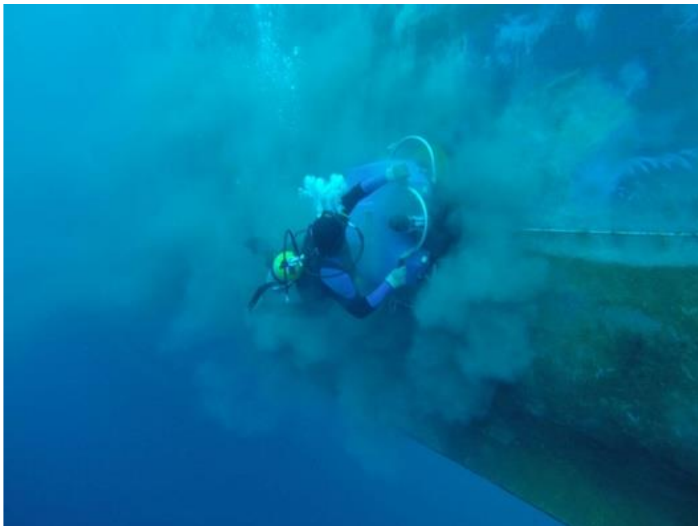
Fig.1: Traditional dust cloud from IWHC without capture
