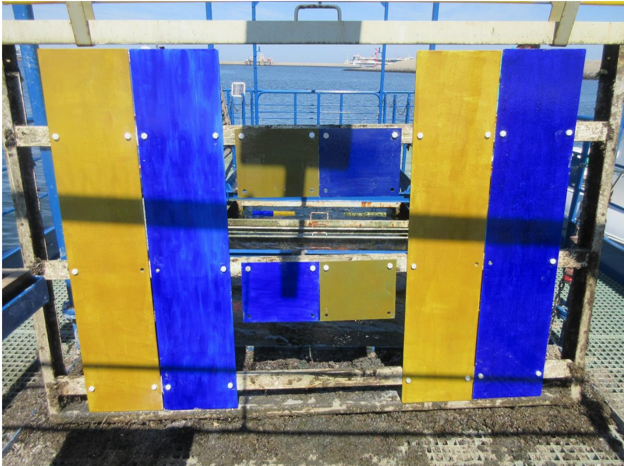
Fig.2: Coated panels mounted on metal frames. Yellow coatings are foul-release, blue coatings are Slips.
