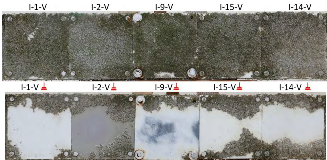
Fig.26: Wear testing (IFAM) at Norderney beachside eulittoral at 4 th inspection on October 20 th , 2020, after 166 days: Top: before cleaning; below: after 30 s cleaning by hard brush.
