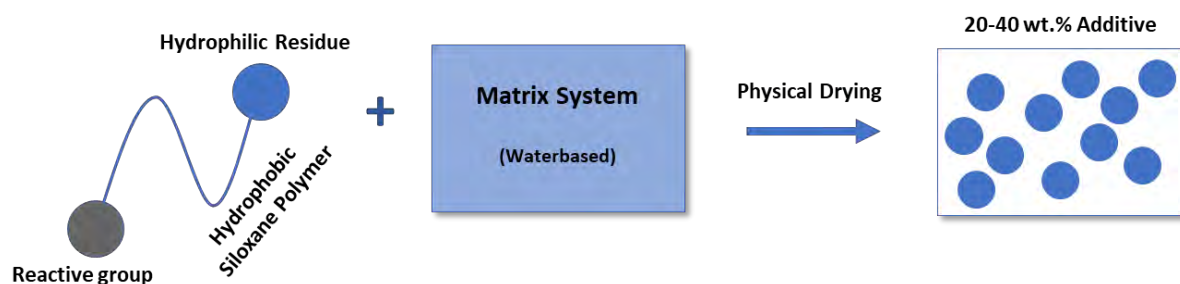
Fig.5: Scheme of physical drying of water-based coatings
