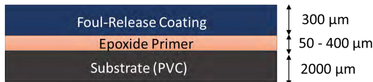
Fig.1: Layered structure of the coating approach (Momentive Performance Materials GmbH)
