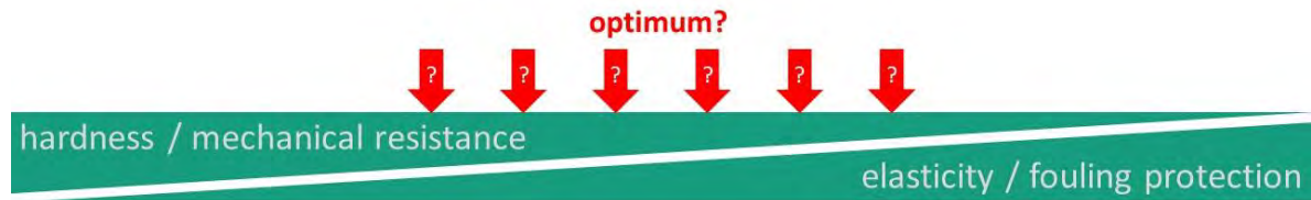
Fig.8: Schematic illustration of the considerations driving the coating development approach of Fraunhofer IFAM in finding an optimum between mechanical robustness without compromising the good fouling release performance of elastomeric materials
