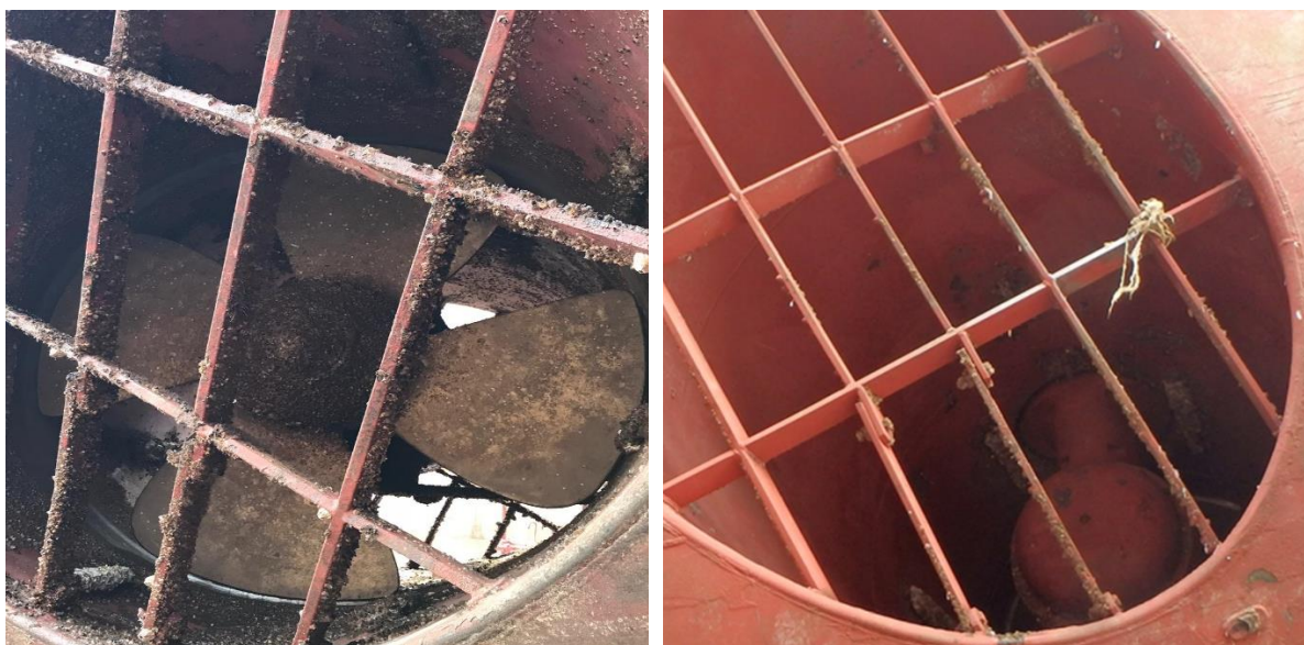
Fig.7: Side thruster before (left) and after (right) installing DBP
