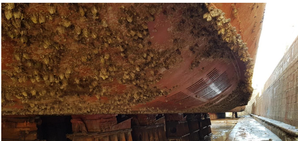
Fig.5: Sea Chest view from outside after 3.5 years in operation with DBP
