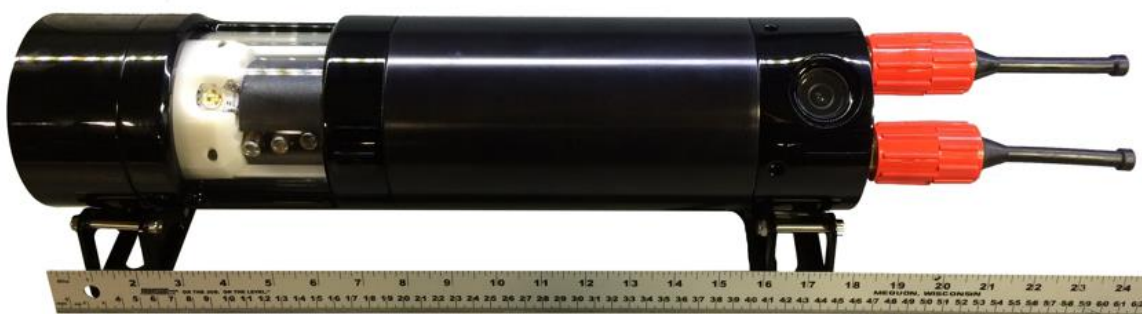
Fig.1: SeaVision™ self-referenced laser scanning system
