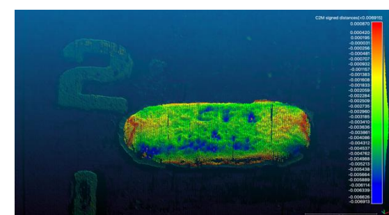
Dimensional coloring to highlight corrosion (light and dark blue) and biofouling (yellow and red) of the anode
