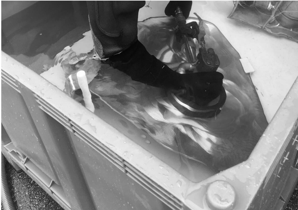
Fig.2: Polishing operation during ex situ test
