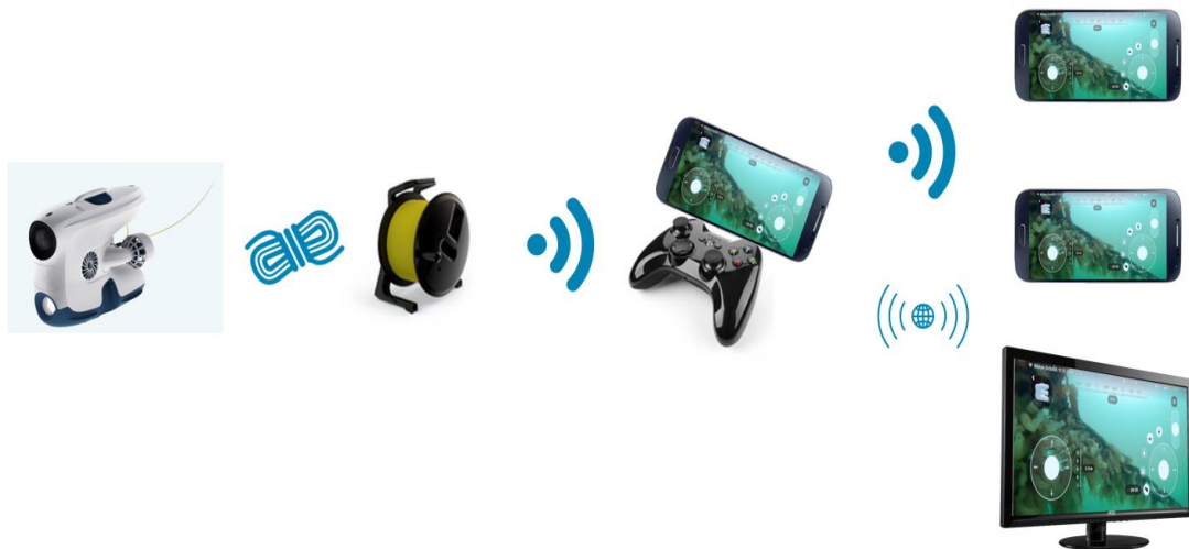
Fig.6: ROV operation framework including streaming via Wi-Fi or internet
