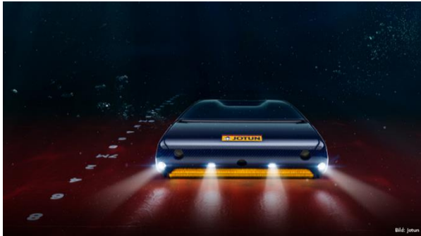
Fig.3: Hull Skater combines inspection and cleaning, source: Jotun
