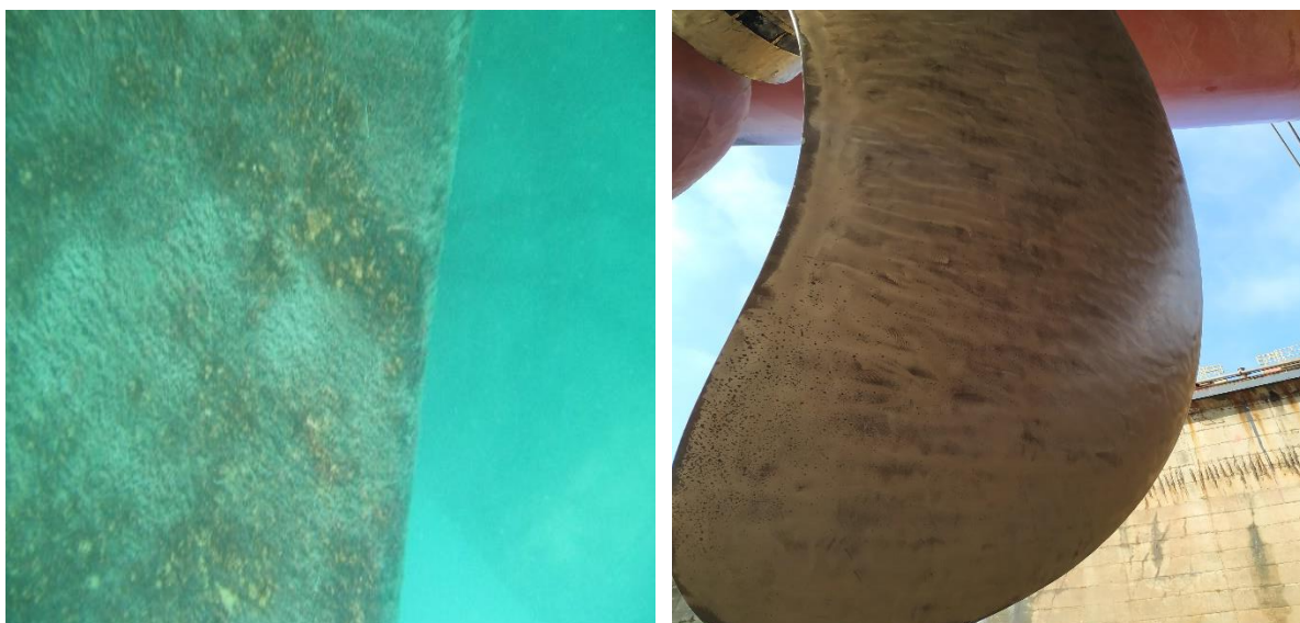
Fig.6: Propeller after 6 months without DBP and comparable propeller after 3 years with DBP
