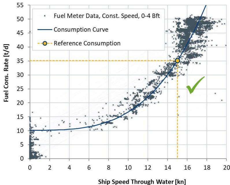
Fig.4: Speed and consumption data from sensors, 10 minutes intervals, same three-month period
