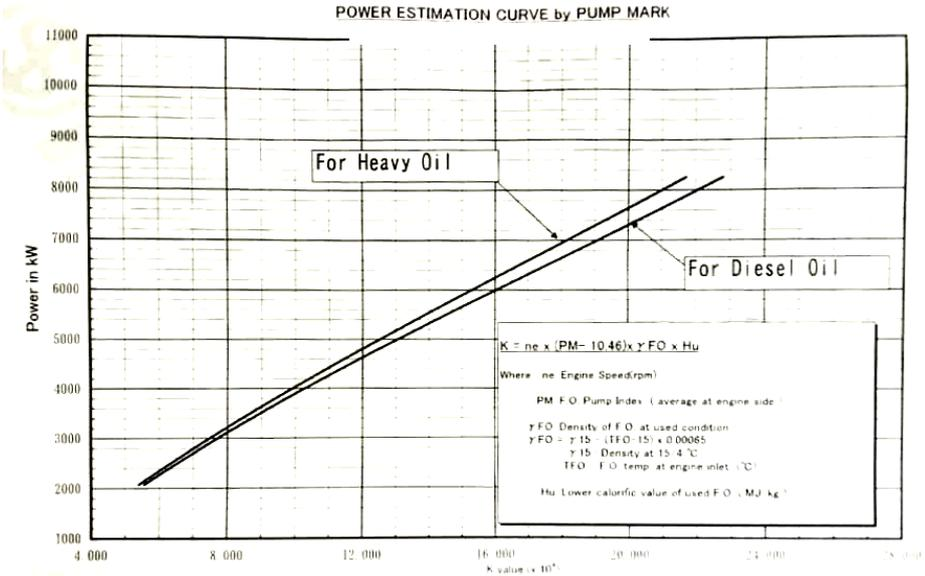
Fig. 11: Power estimation curve example (with FO parameters)
