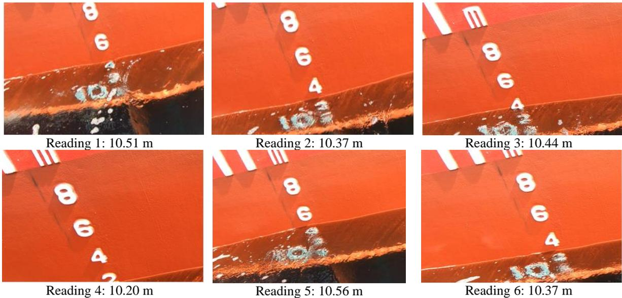
Fig.3: Sample draught measurements after the trials (consequent waves crests and troughs at transom)
