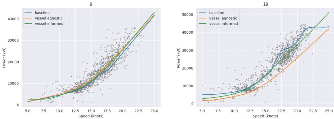
Fig.7: Power vs. Speed for two representative Container ships (left and right) showing actual data (grey dots) and predictions of a vessel specific baseline model trained on the actual data (blue) and vessel agnostic (orange) and vessel informed (green) models trained on other vessels
