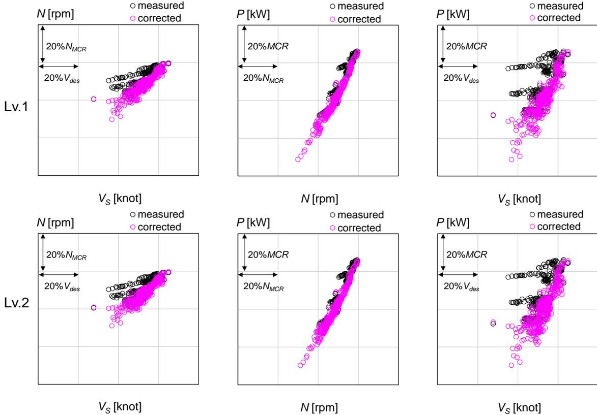
Fig.7: Correction of engine revolution and power. (BC3, upper: Level-1, lower: Level-2)
