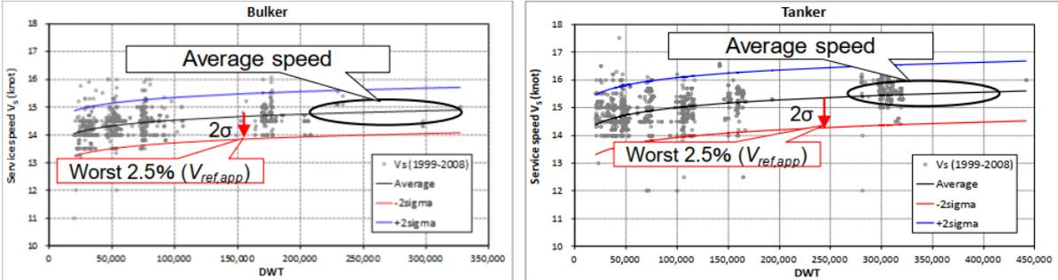
Fig.1: Estimation of  $V_{ref}$  for Bulkers and Tankers
