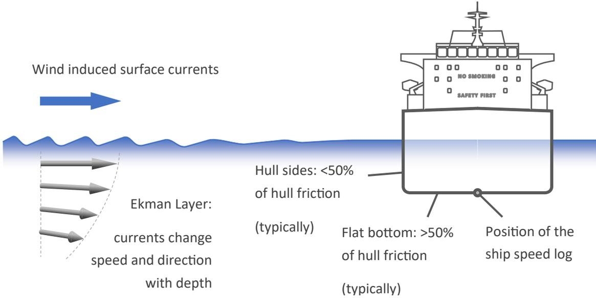
Fig.8: Measuring ship speed through water where hull friction is most relevant
