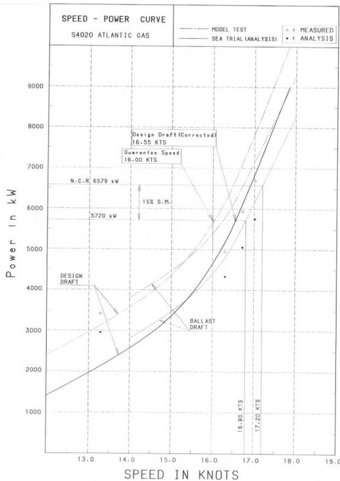
Fig.3: Sea trial results ballast & design – light ballast drafts penalized the performance
