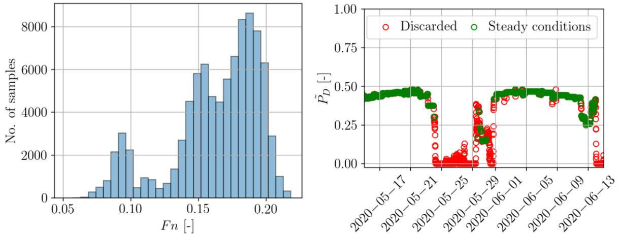
Fig.1: Histogram of the non-dimensional ship speed  $F_n$  based on the filtered dataset (left) and filtering for steady sailing conditions shown for the non-dimensional shaft power  $P_D$  in early 2020 (right)
