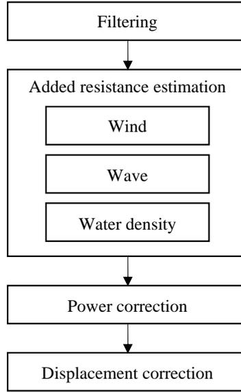
Fig.1: Performance analysis procedure
