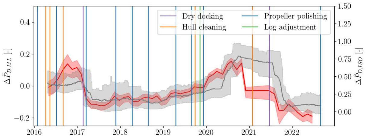
Fig.9: Overlay of the individual 90% prediction intervals derived from ISO 19030 (grey) and the machine learning framework using MC Dropout (red)
