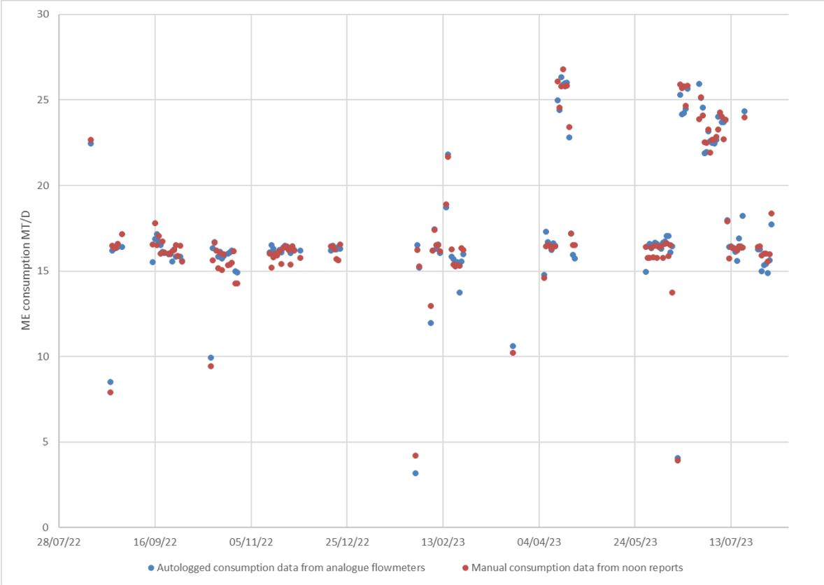
Fig.7: Comparing automated consumption monitoring to noon report data
