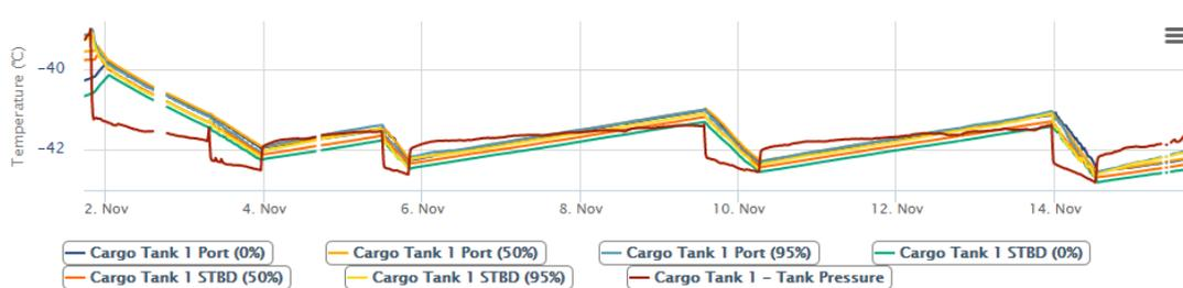
Fig. 9A Standard cooling and correct cooling strategy during longer laden voyages
