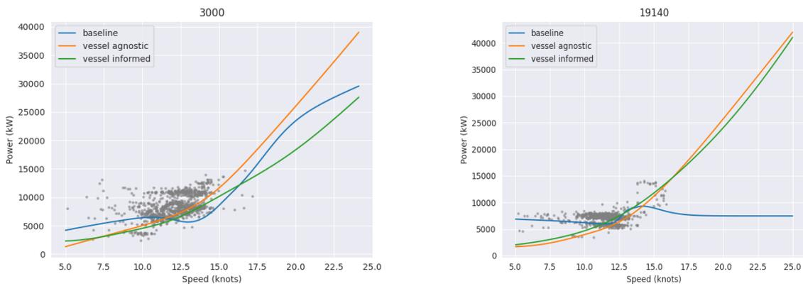
Fig.8: As Fig.7 for two representative Bulk carriers (left and right)
