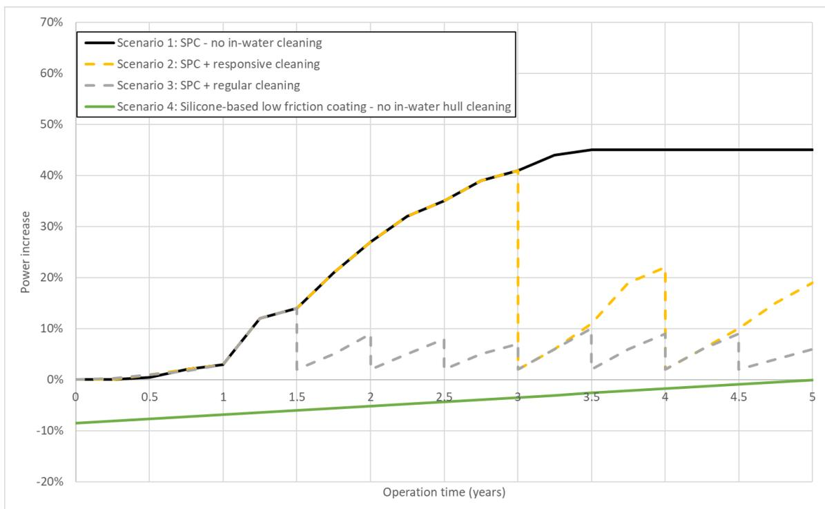
Fig.2: Required power increase of a bulk carrier with different biofouling management strategies over the 5-year operation, adapted from *GEF-UNDP-IMO (2022)*
