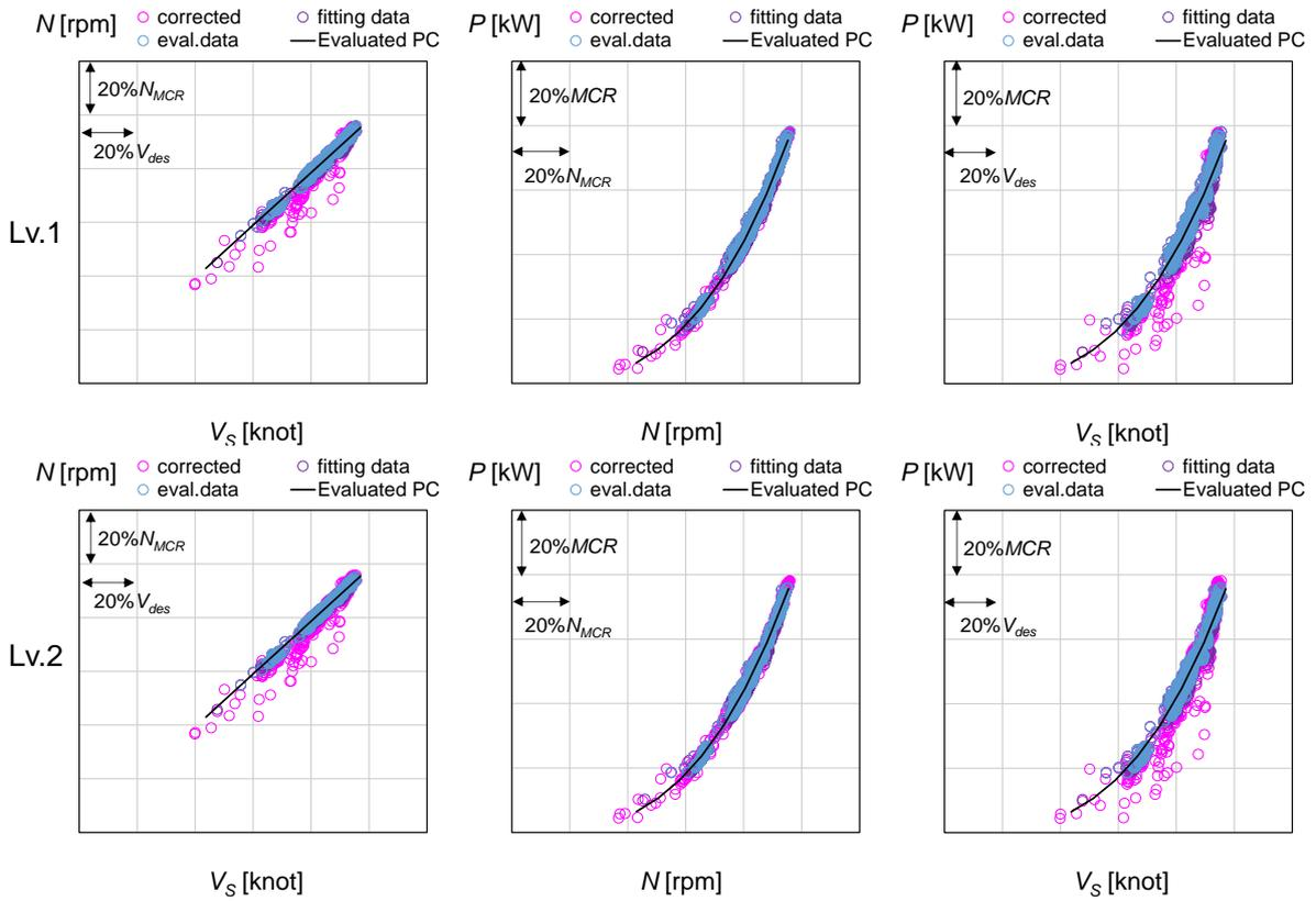
Fig.8 Result of evaluation of ship performance in calm seas. (PCC1, upper: Level-1, lower: Level-2)
