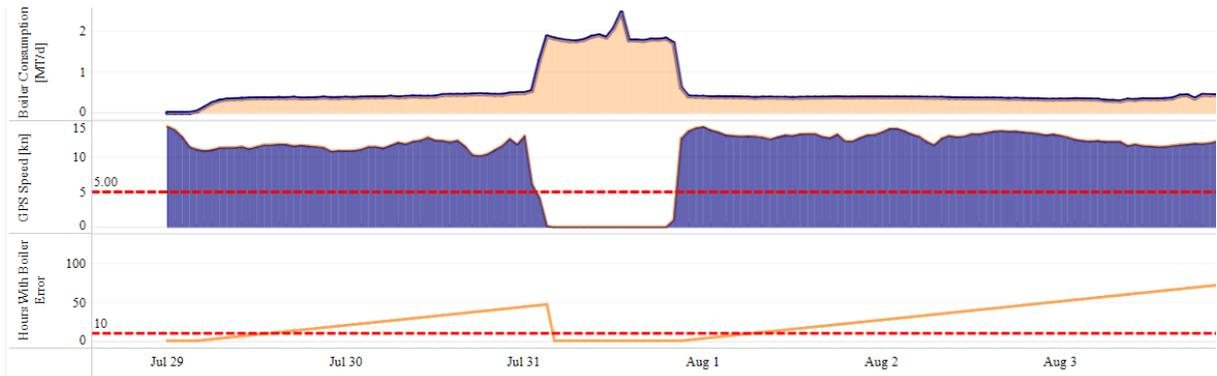
Fig.8: Oil-fired boiler running when main engine is in operation
