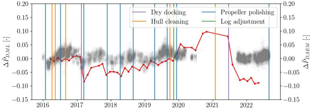
Fig.8: Isolated power increase caused by propeller fouling obtained through machine learning (primary axis) and the results of the semi-empirical framework in transparent grey color (secondary axis)
