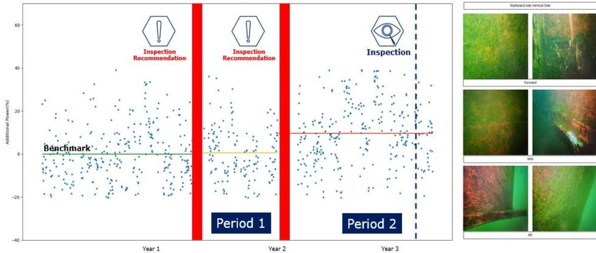
Fig.1: Additional power over time overlapped with suggestions from a predictive fouling risk system
