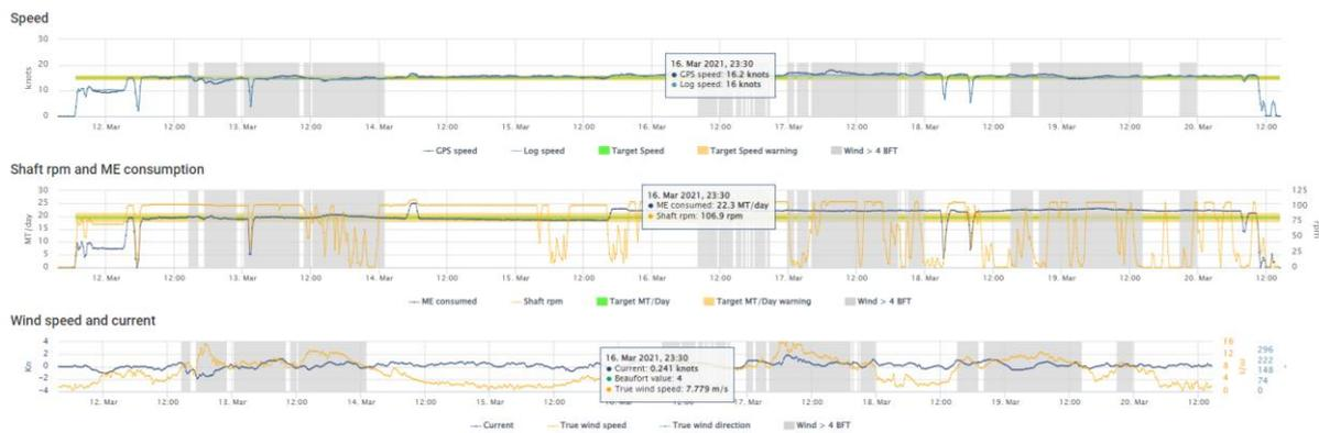
Fig.12: Voyage overview of consumption, speed (log & GPS), shaft rpm, wind speed and current. The shaded areas are time with wind > BF4
