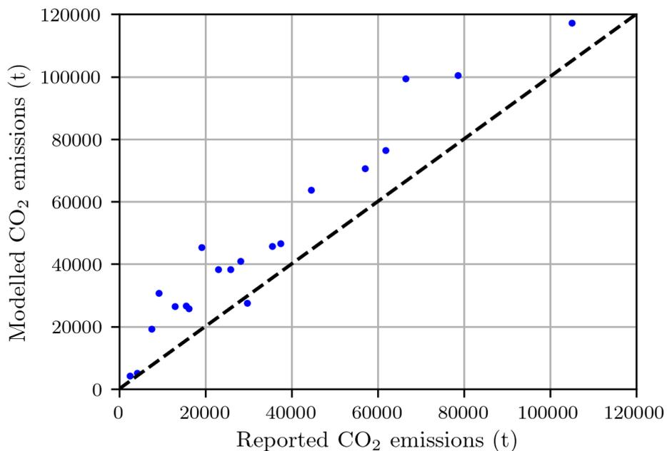
Fig.5: Reported vs. simulated CO<sub>2</sub> –emissions for year 2021 for 20 vessels.
