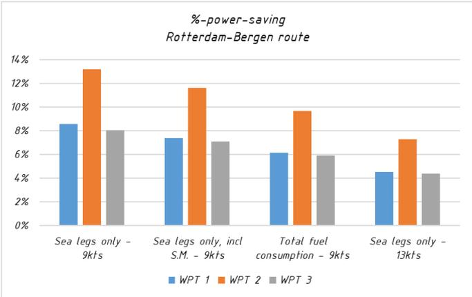
Fig.4: Percentage power saving can be computed in different ways, and for different conditions, which results in different performance expectations
