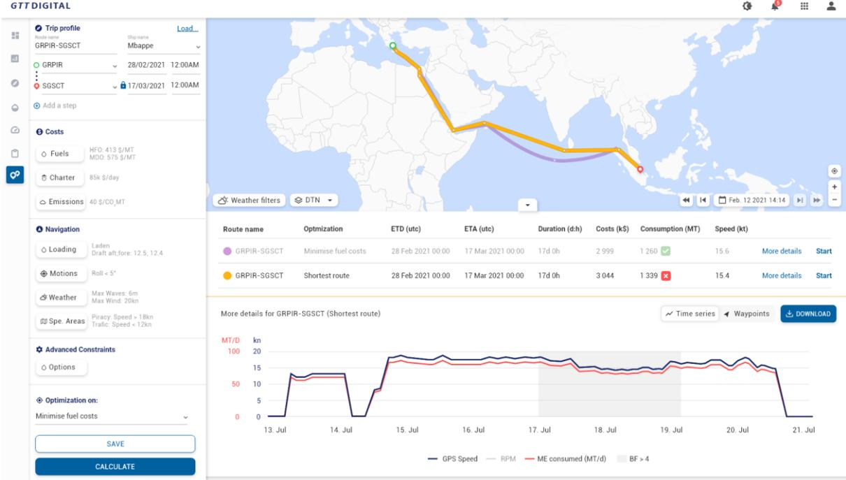
Fig.20: Example of a voyage-based route optimization integrated in the performance system
