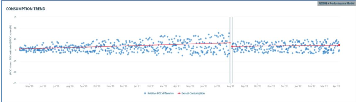
Fig.1: Effect of fouling and maintenance show in the consumption trend graph
