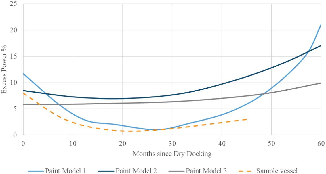
Fig.2: Comparison of different paint models and a sample vessel
