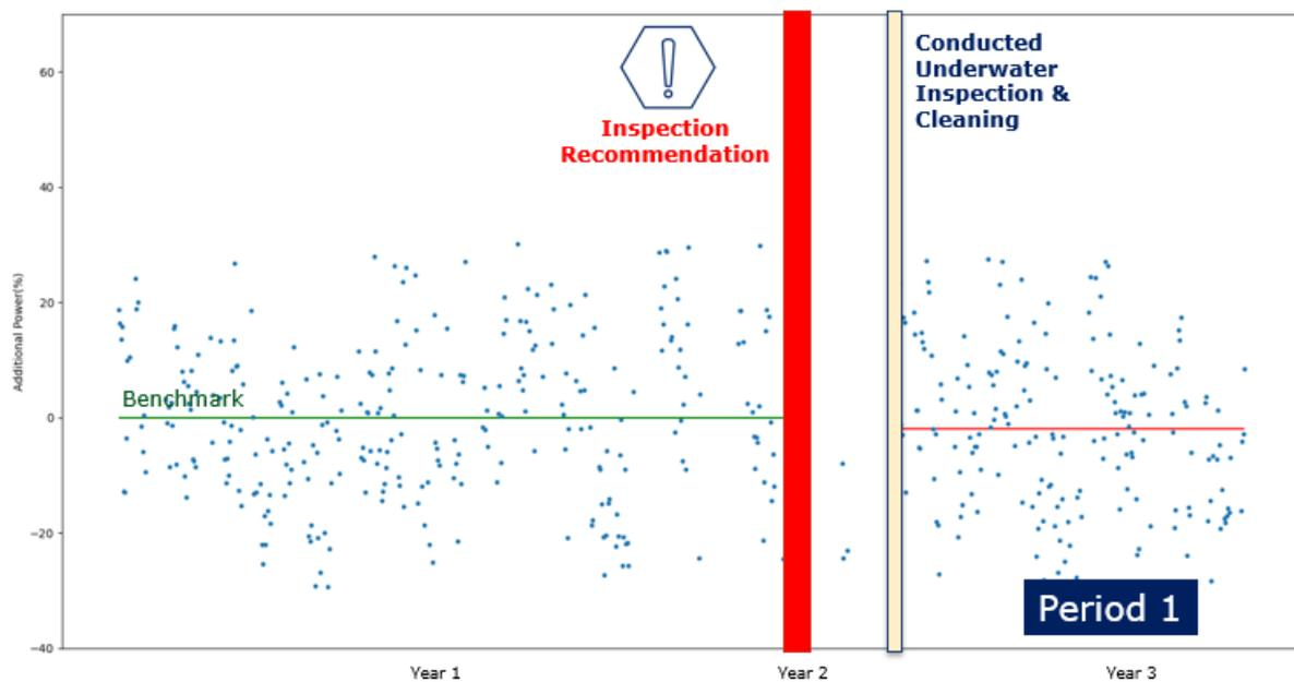
Fig.2: Additional power over time overlapped with suggestions from a predictive fouling risk system
