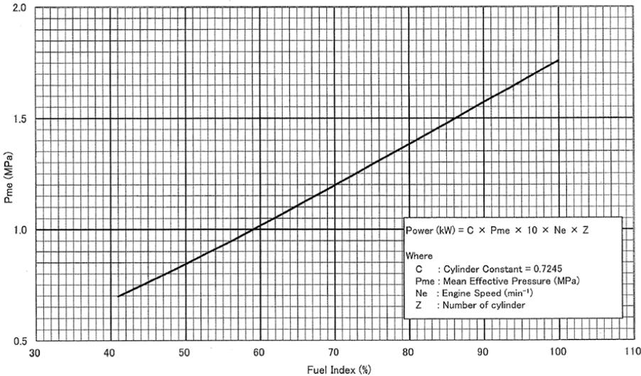
Fig. 10: Power estimation curve example (Pme only)
