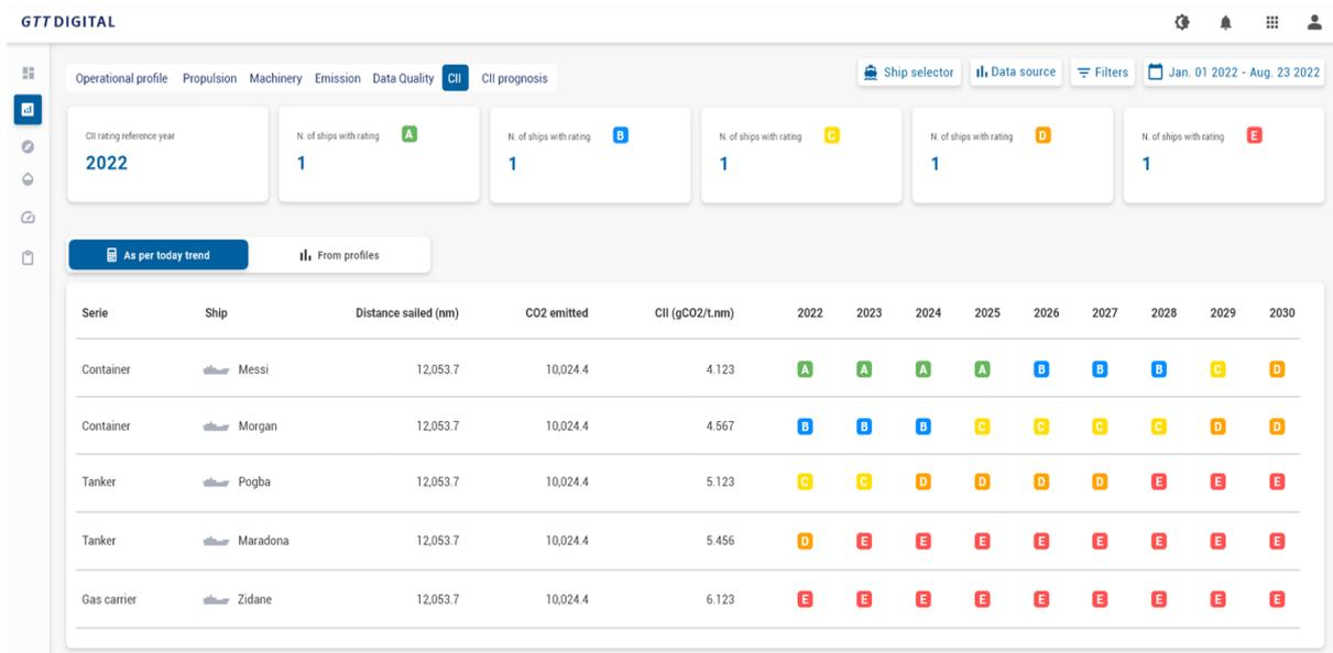
Fig.23: Fleet CII overview tool based on current performance and operational profile
