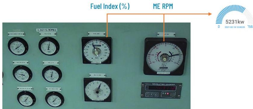
Fig. 12: Live monitoring and calculation of engine power on MC engines
