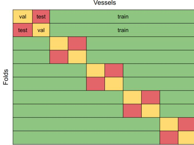
Fig.4: Illustration of the ten-fold cross-validation methodology. The vessels are divided into five folds (A, B, C, D, E) each subdivided into two sub-folds (i and ii). Each of the experiments reported in this paper is run by first training on B-E, validating on Ai and testing on Aii, then training on B-E, validating on Aii and testing on Ai, then training on A, C-E, validating on Bi and testing on Bii etc. Reported results are the average of all the sub-fold tests.
