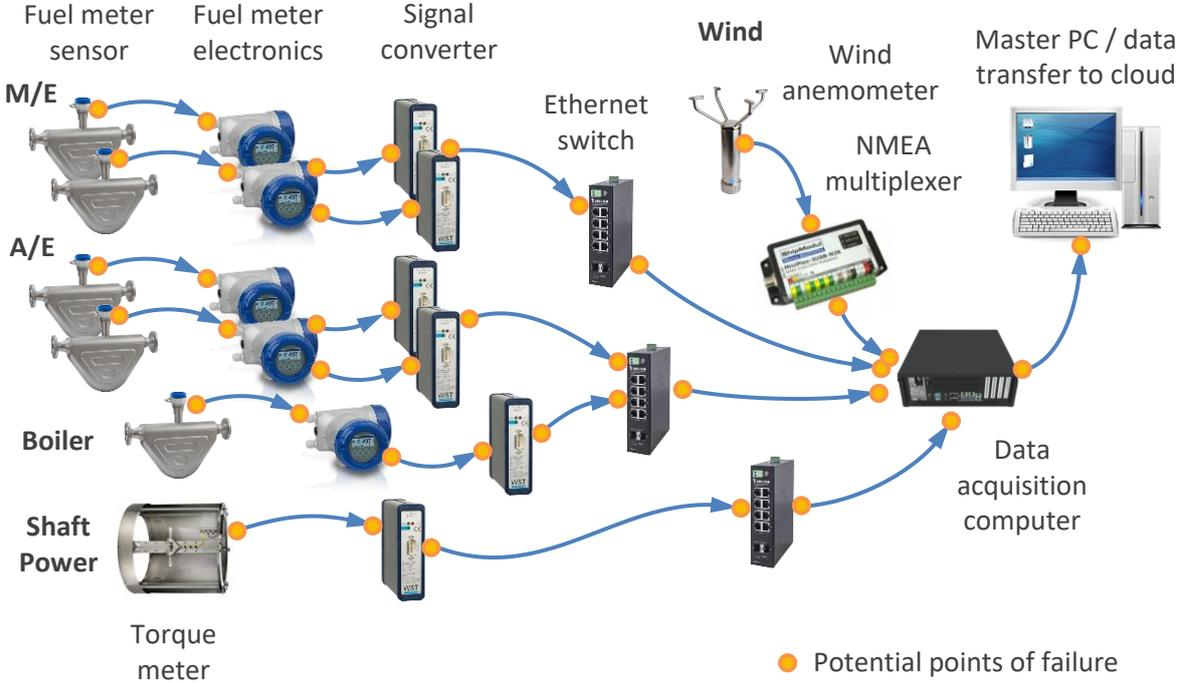
Fig.5: Multiple electronic devices and connections create a large number of potential points of failure
