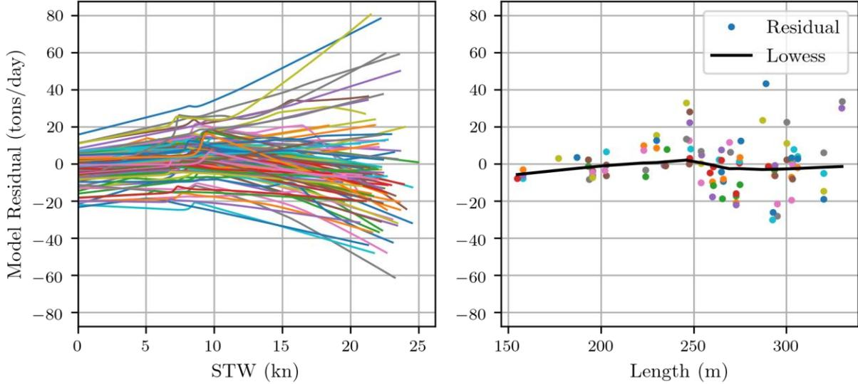
Fig.2: Left: LOWESS plots of the model residuals as a function of speed through water for each of the  $N=98$  vessels. Right: The average model residual for each vessel as a function of vessel length.
