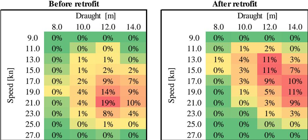
Fig.4: Operational profile of a large container vessel before retrofit (left) and after retrofit (right)
