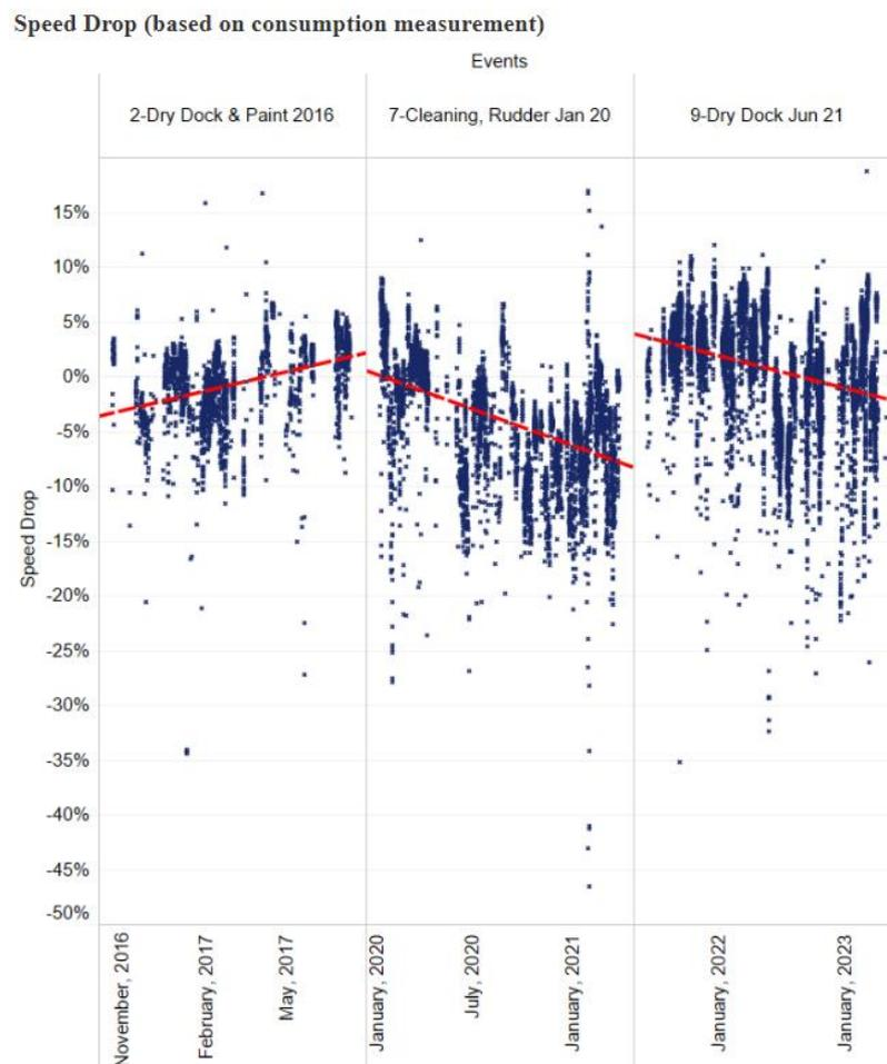
Fig.6: Consequence on performance from increased idling and lack of cleaning
