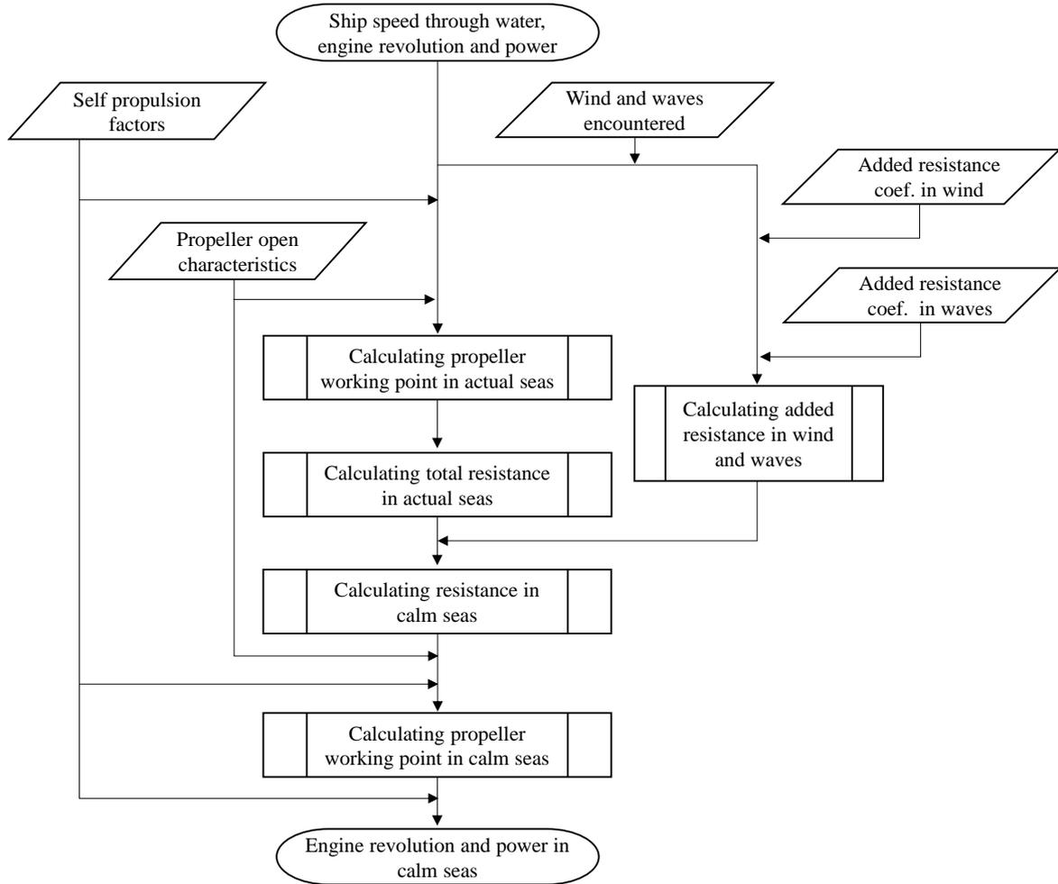
Fig.4: Flowchart of correction of engine revolution and power
