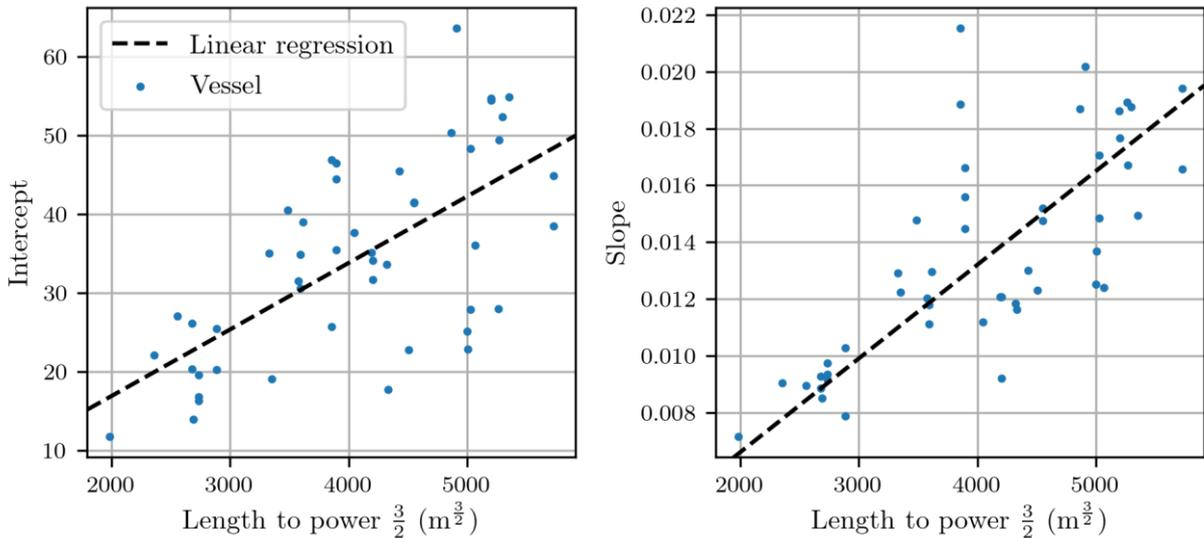
Fig.1: Parameters  $a_i$  (intercept) and  $b_i$  (slope) estimated from Eqs.(5) and plotted against vessel length to the power  $k = \frac{3}{2}$  for a sample of  $N = 98$  cruise vessels.
