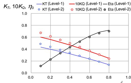
Fig.2: Propeller open characteristics
