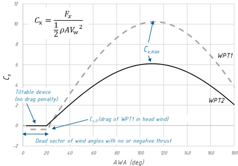
Fig.2: Example characteristics of WPTs, illustrated as thrust force coefficient ( $C_x$ ) vs. apparent wind angle (AWA) curves for two different WPTs
