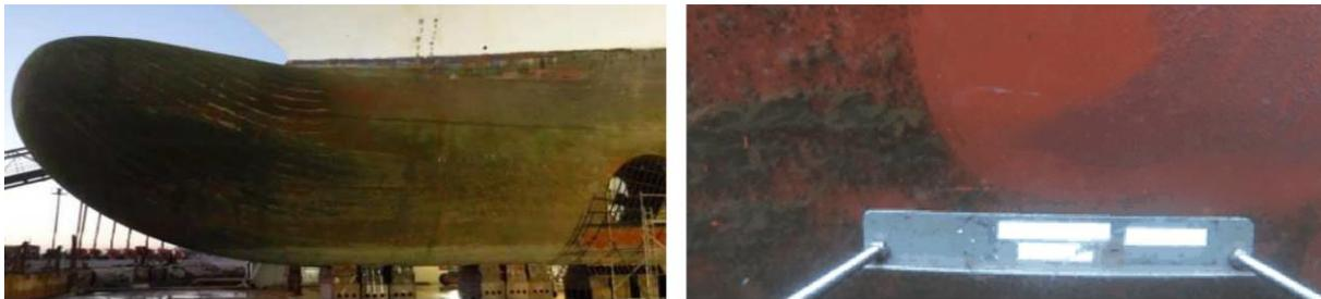
Fig.5: Visual appearance of the bulbous bow in February 2017 after almost 5 years since the last dry-docking (left) and effect of the robotic in-water cleaning on a vertical wall in early 2021 (right)
