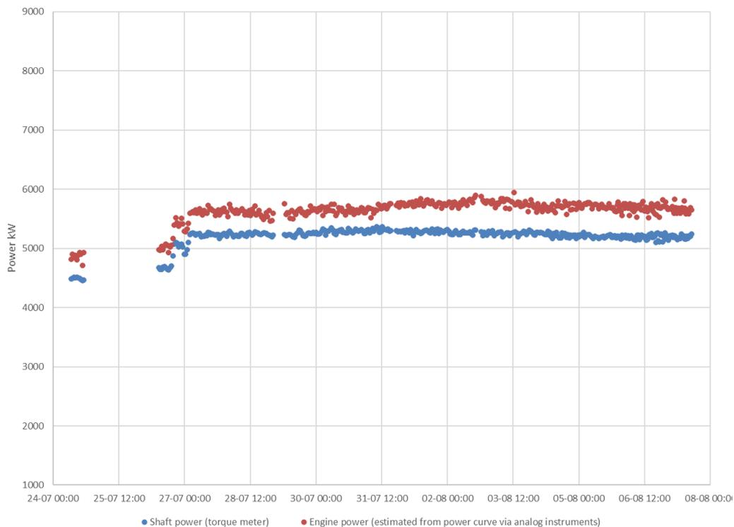
Fig.13: Comparing engine power to shaft power
