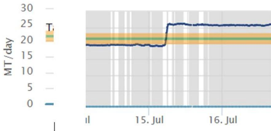
Fig.5: Increase of consumption due to fuel oil shifting from forward to aft increasing aft trim
