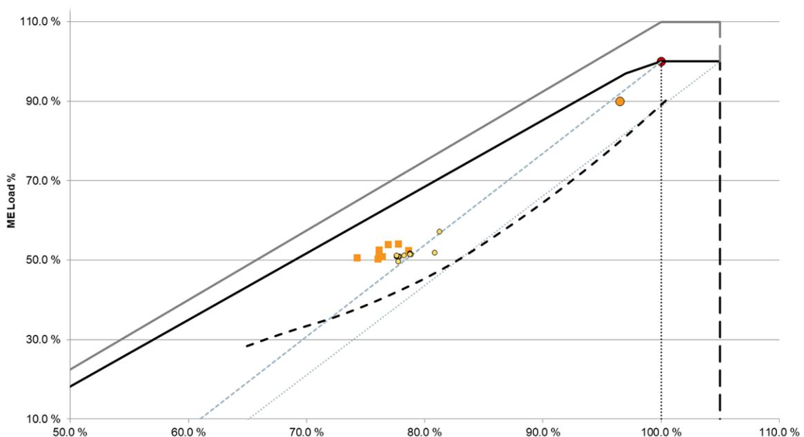
Fig.1: Main engine diagram with operational data and Design Propeller curve (before & after installing a pre-swirl device)
