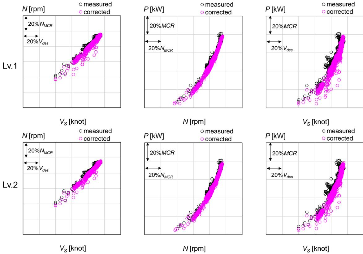
Fig.6 Correction of engine revolution and power. (PCC1, upper: Level-1, lower: Level-2)
