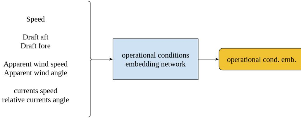
Fig.2: Architecture of the operational encoder network, used to obtain a vector embedding representing the operational conditions of the vessel at each point in time. The light blue square represents trainable neural network layers.
