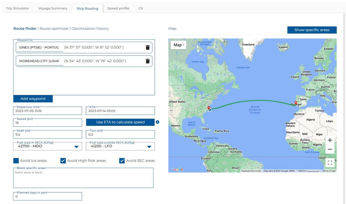
Fig.2: Main view of SeaPerformer when planning a route
