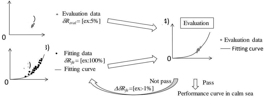
Fig.5: Outline of evaluation by increase rate of added resistance
