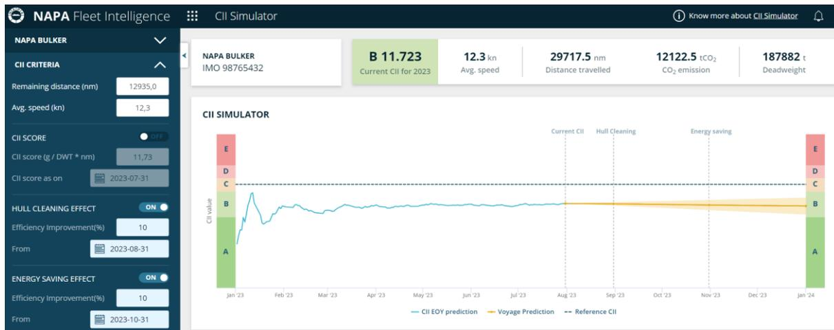
Fig.3: Example of CII prediction assimilating information about planned maintenance and installation of energy saving devices
