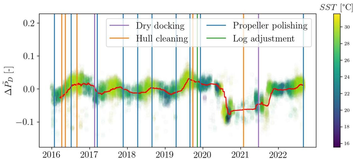
Fig.7: Result of semi-empirical framework including the sea surface temperature in the colorbar and a 30-day rolling mean in red. It is noted that no filtering thresholds are applied to the forward speed.
