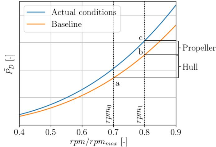
Fig.2: Contribution of hull and propeller performance for two different conditions considering shaft rpm vs. shaft power, according to *Park et al. (2018)*
