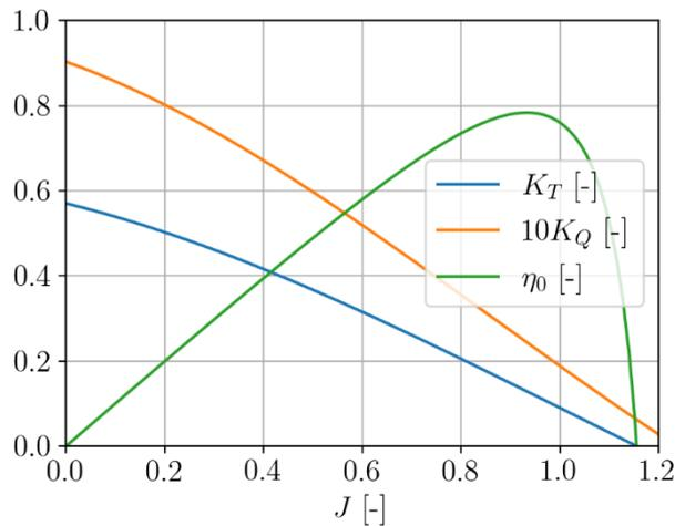
Fig.3: Full-scale open-water propeller curves according to the Wageningen B series for an FPP with  $D=5.8\text{m}$ ,  $A_E/A_0=1.05$ ,  $P/D=1.1$  and  $Z=6$ .  $A_E/A_0$  is the expanded blade area ratio and  $P/D$  the pitch diameter ratio. Only public-domain information about the vessel was used.
