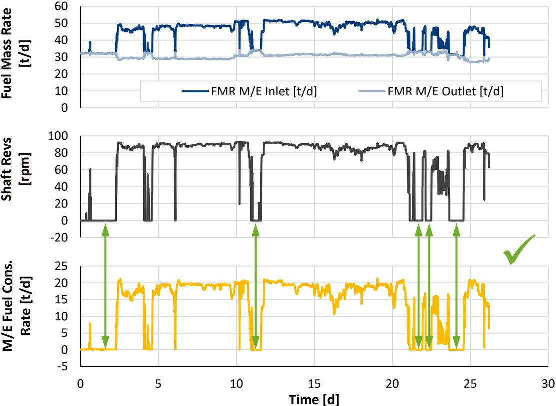
Fig.7: Exemplary vessel data showing when the correct functioning of the fuel meters can be checked
