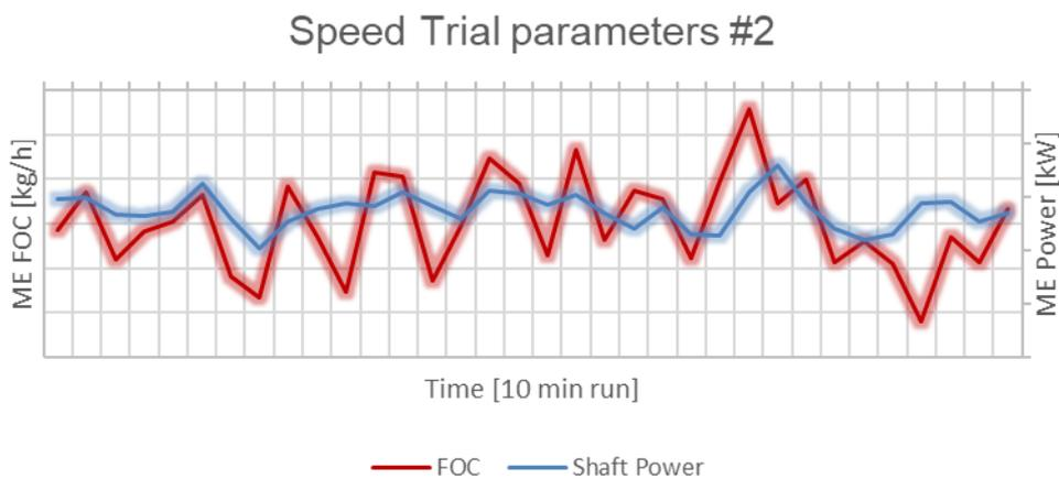
**Fig.5: Sample Power and Fuel Oil Consumption values**
