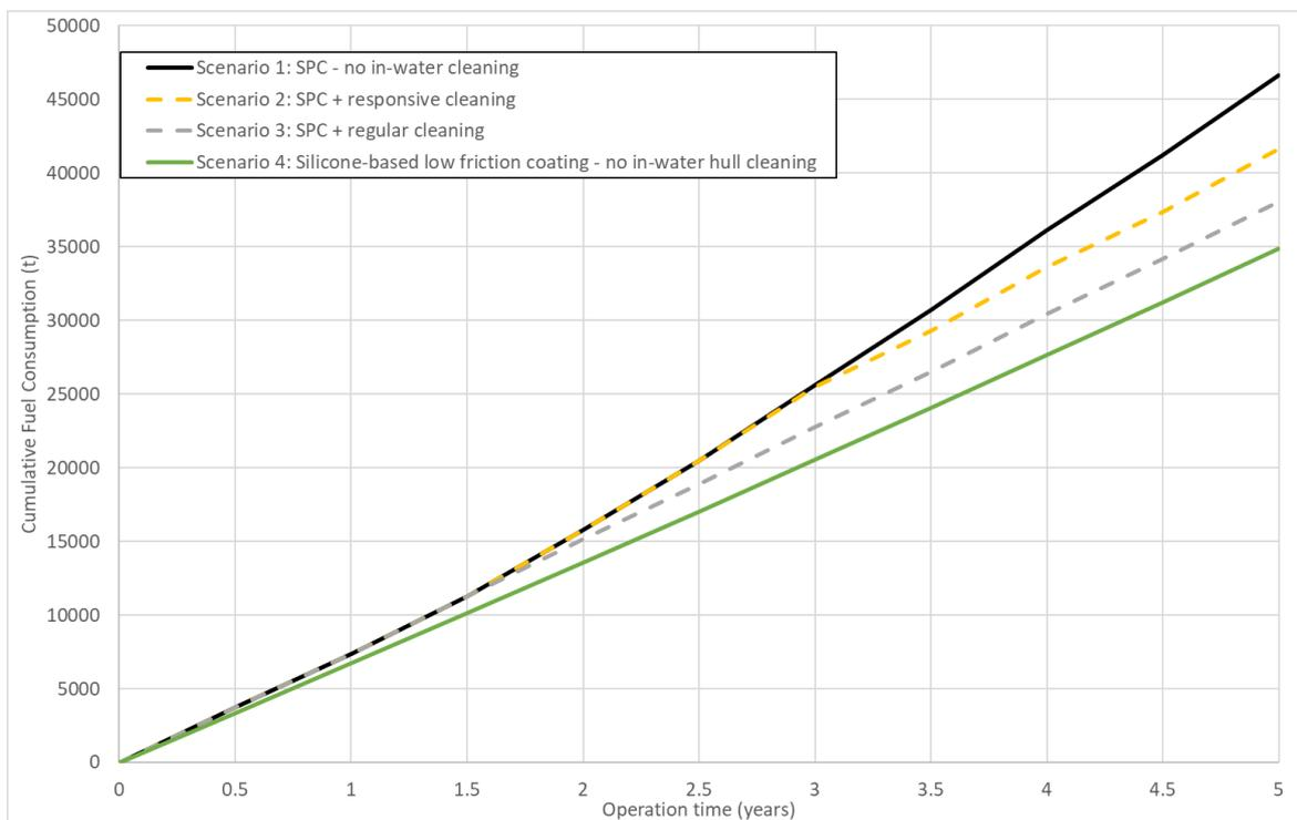
Fig.3: Cumulative fuel consumption of the bulk carrier with different biofouling management strategies over the 5-year operation, adapted from *GEF-UNDP-IMO (2022)*
