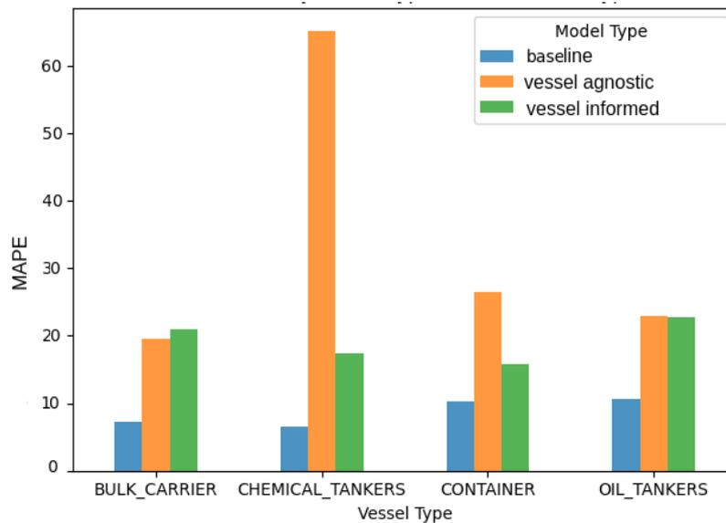
Fig.5: MAPE of predicting power for each vessel type of a model using only operational conditions trained on data from the vessel (blue), a model using only operational conditions trained on data from other vessels (orange) and a vessel informed model using operational conditions, vessel type and hull geometry trained on data from other vessels.
