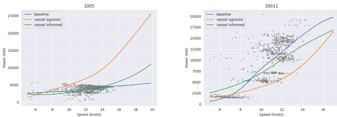
Fig.9: As Fig.7 for two representative tankers (left and right)
