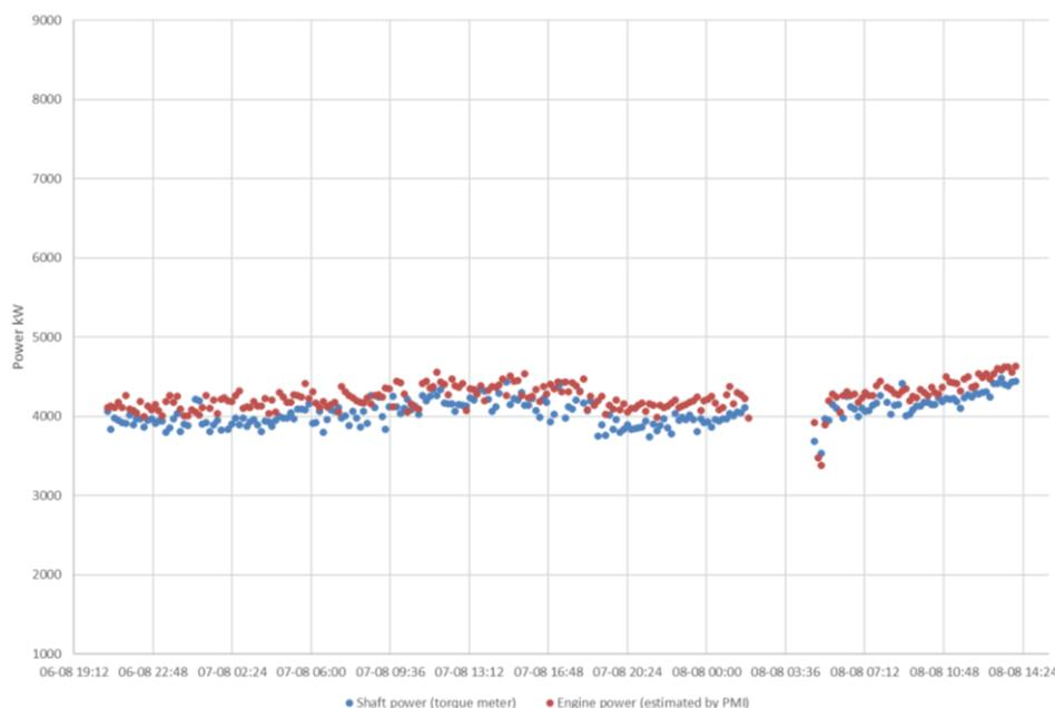
Fig. 9: Comparing engine power (from PMI) to shaft power for an electronically controlled engine
