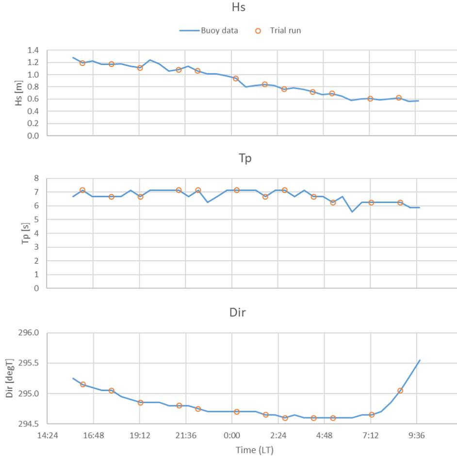
Fig.5: Wave buoy data (wave height, period, direction)
