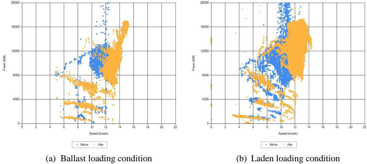
Fig.5: Performance analysis results of vessel C before and after hull cleaning and propeller polishing
