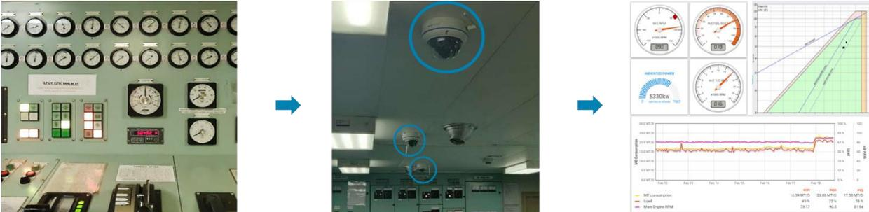
Fig.2: Data collection from analog equipment using AI powered cameras
