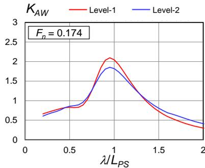
Fig.1: Added resistance in regular waves
