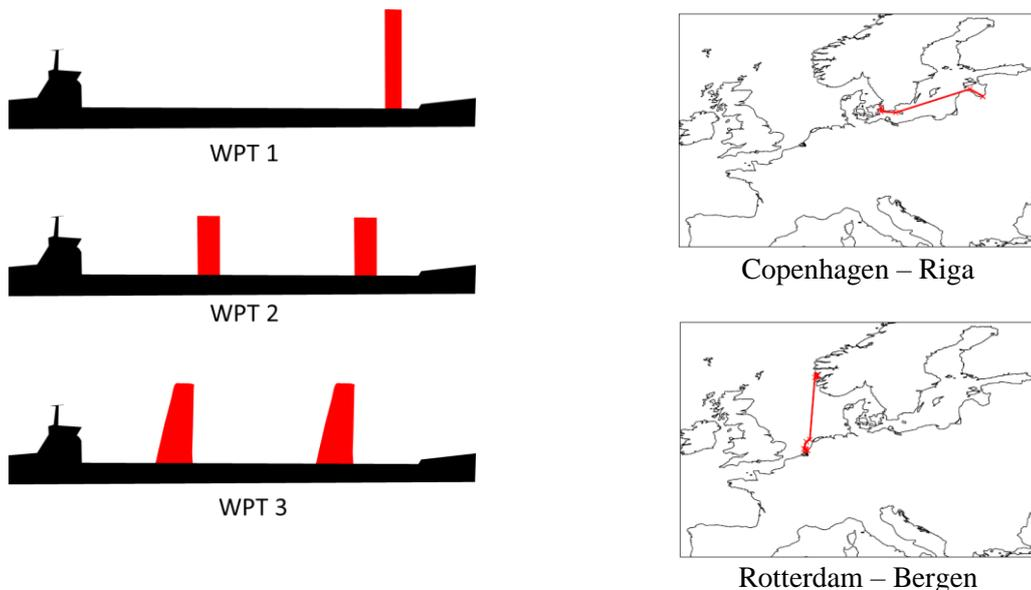
Fig.1: Generic Wind Propulsion Technologies fitted to a general cargo vessel
