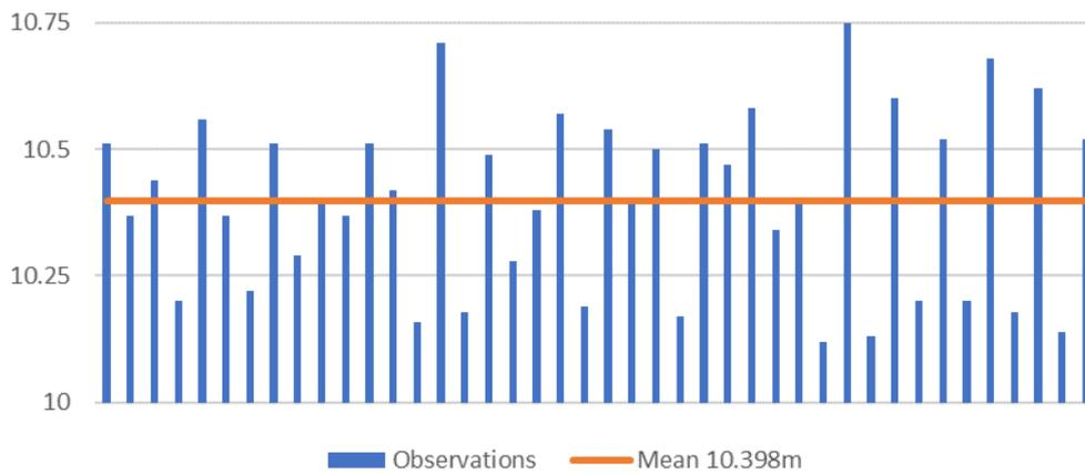
Fig.4: Deriving the mean draught at the transom by averaging consequent waves crests and troughs
