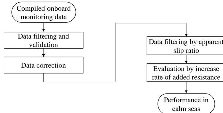
Fig.3: Flowchart of the evaluation model established by the OCTARVIA project.
