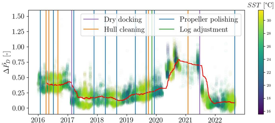
Fig.4: Power increase according to the ISO 19030 procedure with sea surface temperature (SST) in the colorbar and a 30-day rolling mean in red
