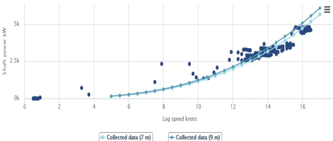
Fig.13: Actual good weather performance vs standard ballast- & laden curves
