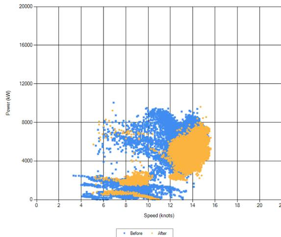
Fig.2: Performance analysis results of vessel A before and after hull cleaning and propeller polishing in ballast loading condition
