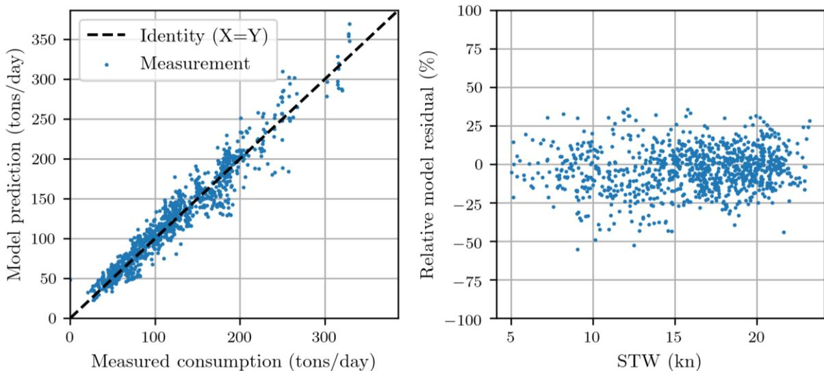
Fig.3: Left: Measured vs modeled consumption of 1000 randomly sampled data points with STW over 5 kn from test data set. Right: Relative residual of fuel consumption as a function of vessel speed.
