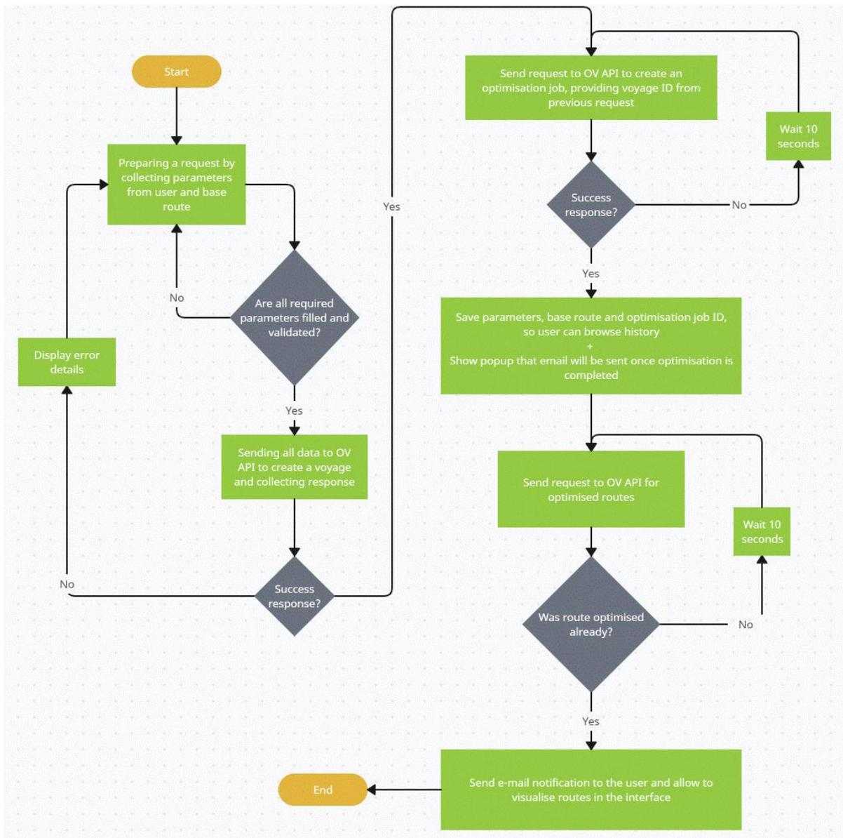
Fig. 1: Data flow chart for SeaPerformer and OV
