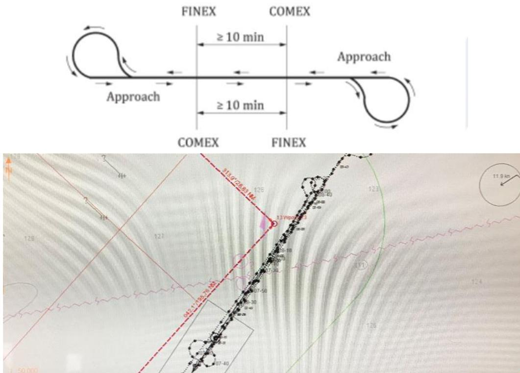
Fig.4: Double run scheme plotted on the ECDIS
