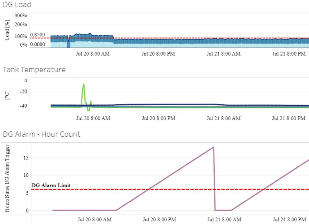
Fig.7: Two diesel generators running at low load (< 85%MCR of one)
