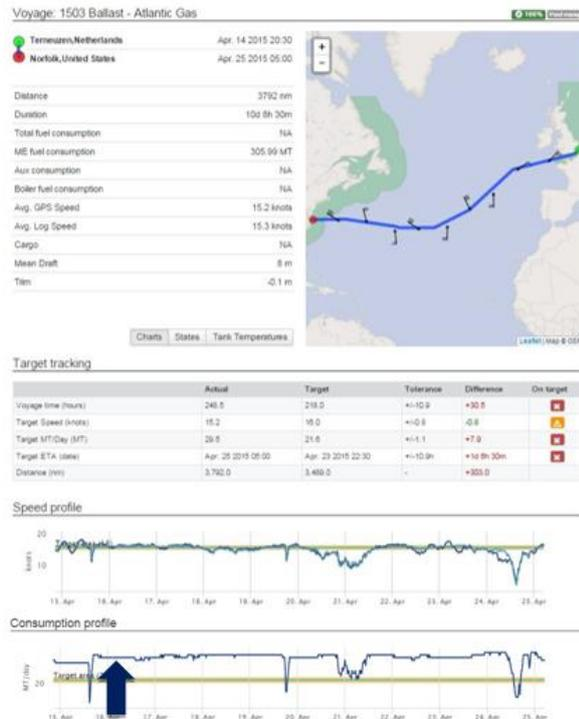
Fig.14A: The consequences of being off voyage target
