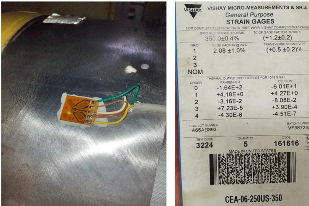
Fig.2: On of the two strain gauges installed on the shaft
