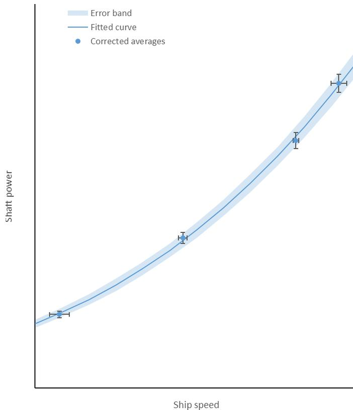
Fig.6: Corrected trial results with error bars per run set and shaded bandwidth around obtained speed/power relation
