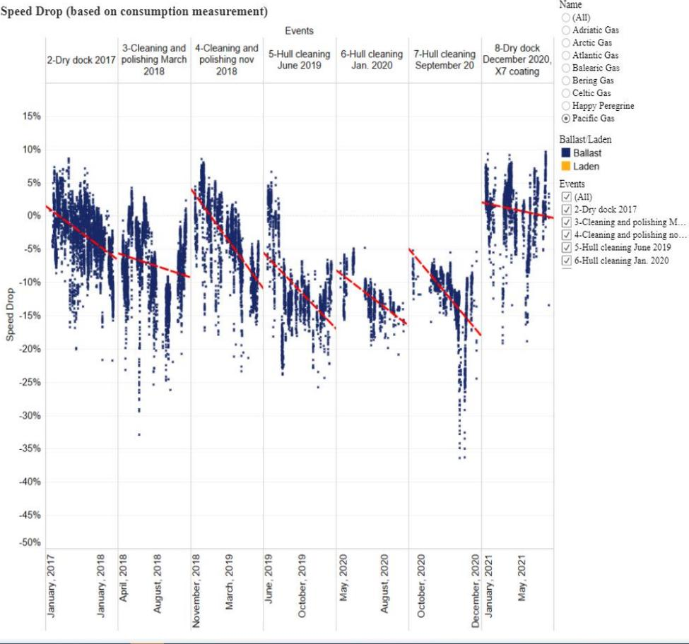
Fig.19: Speed drop over a period of four years until new anti-fouling was introduced
