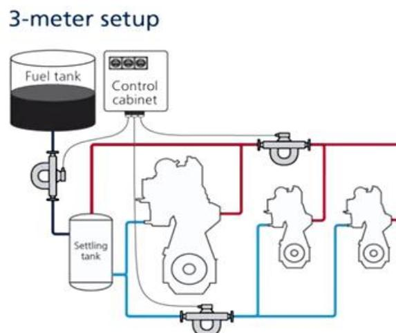
Fig.1: Common (or mono) fuel system. Marine Fuel Flow Meter, Consumption Systems & Measurements, Insatech Fuel Consumption System
