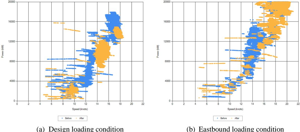
Fig.3: Performance analysis results of vessel B before and after propeller polishing
