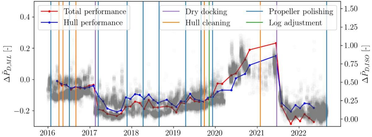
Fig.6: Comparison of the model estimates of the power increase (primary axis) to ISO 19030 results in transparent grey color (secondary axis)
