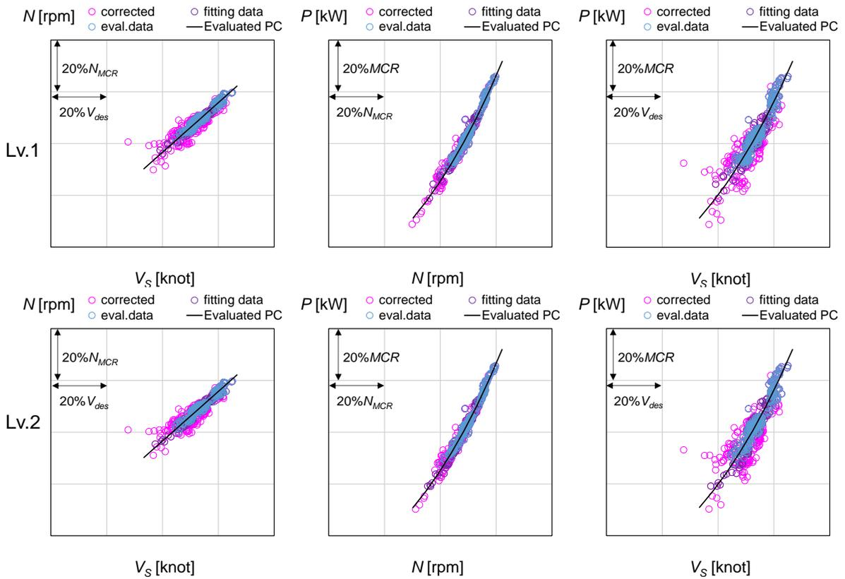
Fig.9: Result of evaluation of ship performance in calm seas. (BC3, upper: Level-1, lower: Level-2)
