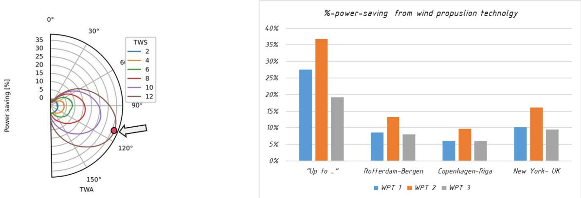
Fig.3: Sometimes the performance is expressed as “up to xx%”, meaning the performance at the most favourable wind condition. The averaged wind condition on a route gives quite different saving.
