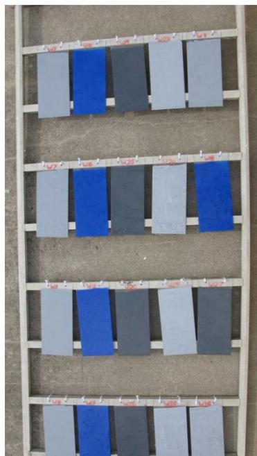
Fig.16: Reference silicon epoxy-coated test panels submerged in April 2016 off the west coast of Sweden.
