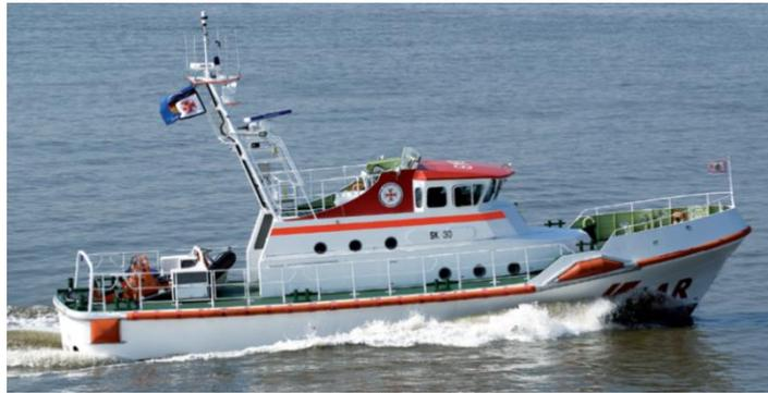
Fig.4: SAR vessel of the German Maritime SAR Association DGzRS (source: fassmer.de). The FLIPPER coatings were designed for a 1:3.2 scale model of this ship (5.72 m length). HSVA thanks the Fassmer group and DGzRS for their permission to use the hull geometry in FLIPPER
