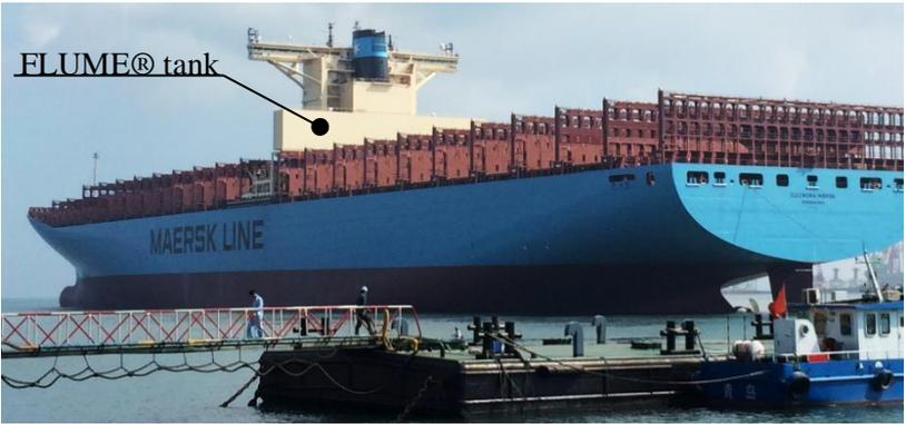
Fig.3: FLUME Tank on a modern Container Ship
