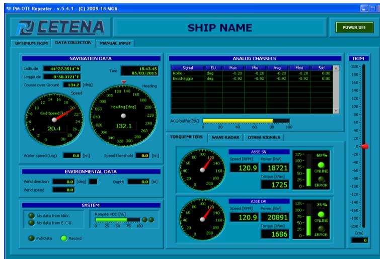
Fig.3: Data collector module
