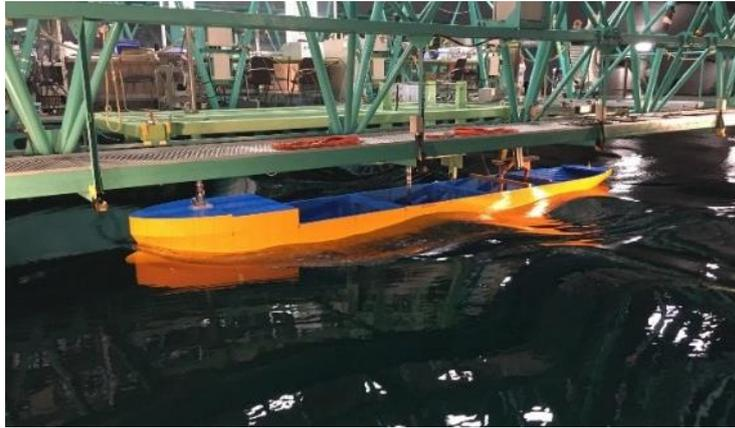
Fig.2: Test in waves of a bulk carrier model at a towing tank
