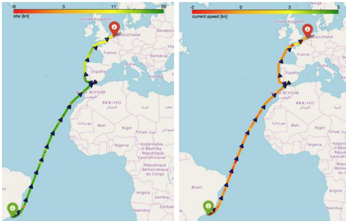
Fig.4: Vessel service route with measured speed-through-water (left) and sea current speed (right)
