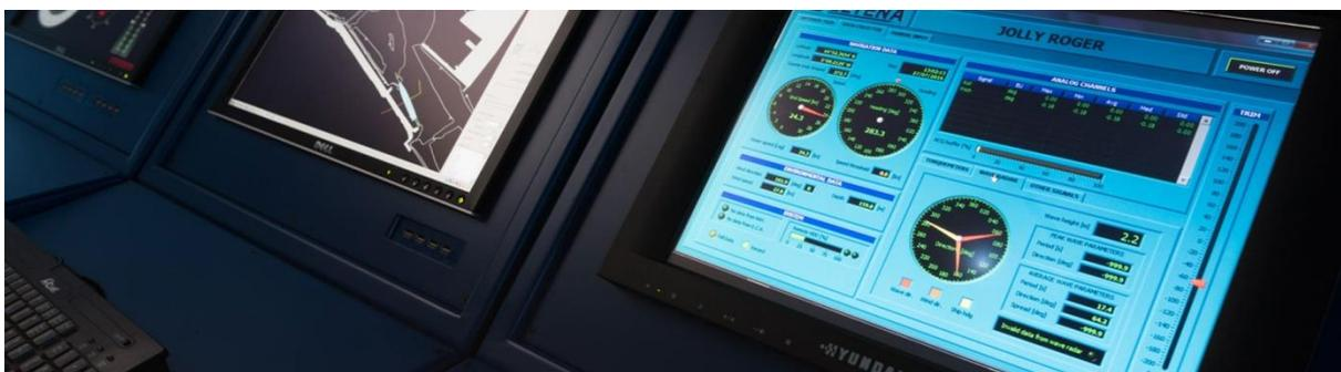
Fig.1: Performance Monitoring arrangement on wheelhouse console
